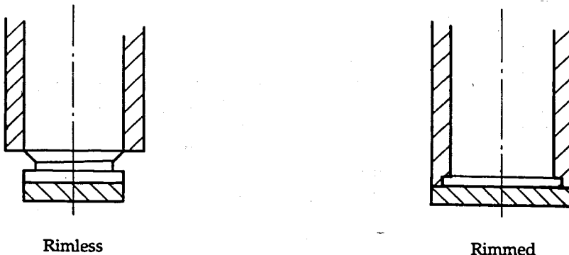
Fig 3.3 Types of Rim and how they are Supported
