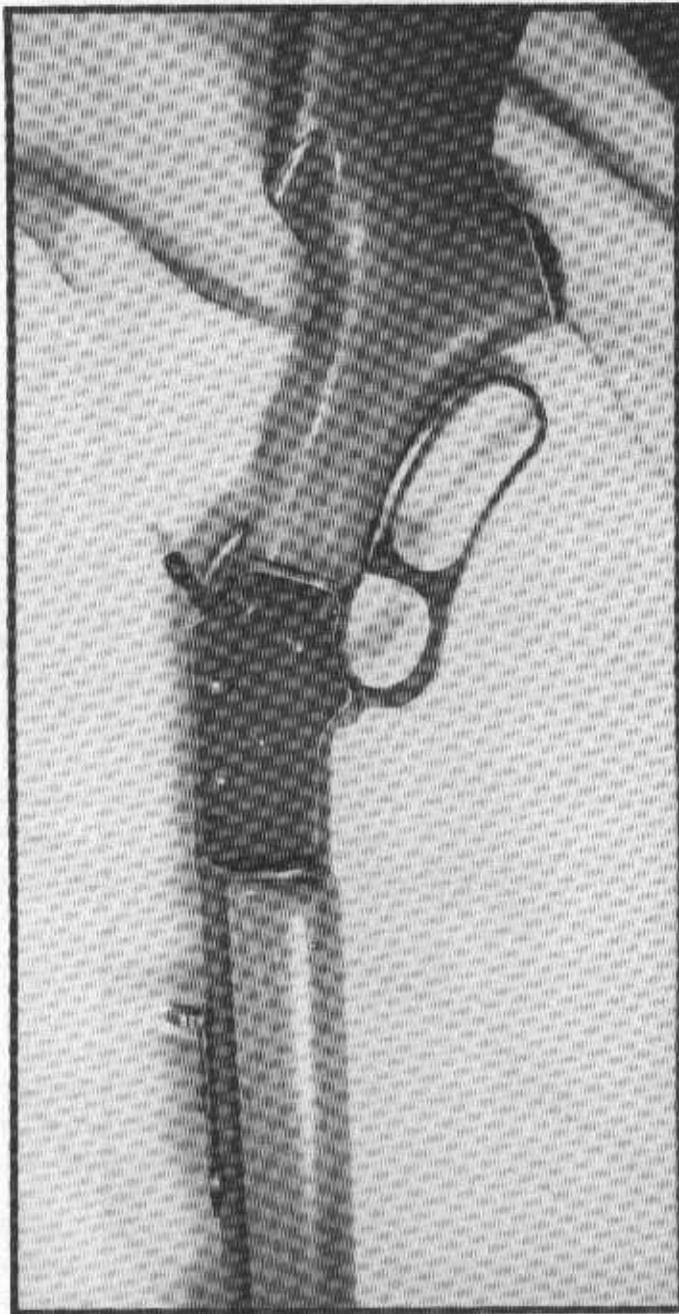
Figure 2-5 The lever action.
