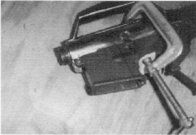
Shop-built upper, clamped to commercial lower with bushing in front pin hole, ready for drilling.
