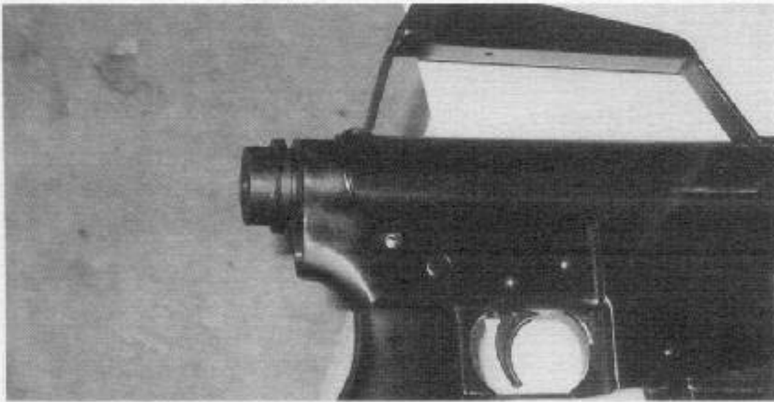
Breech plug partially screwed in place.
