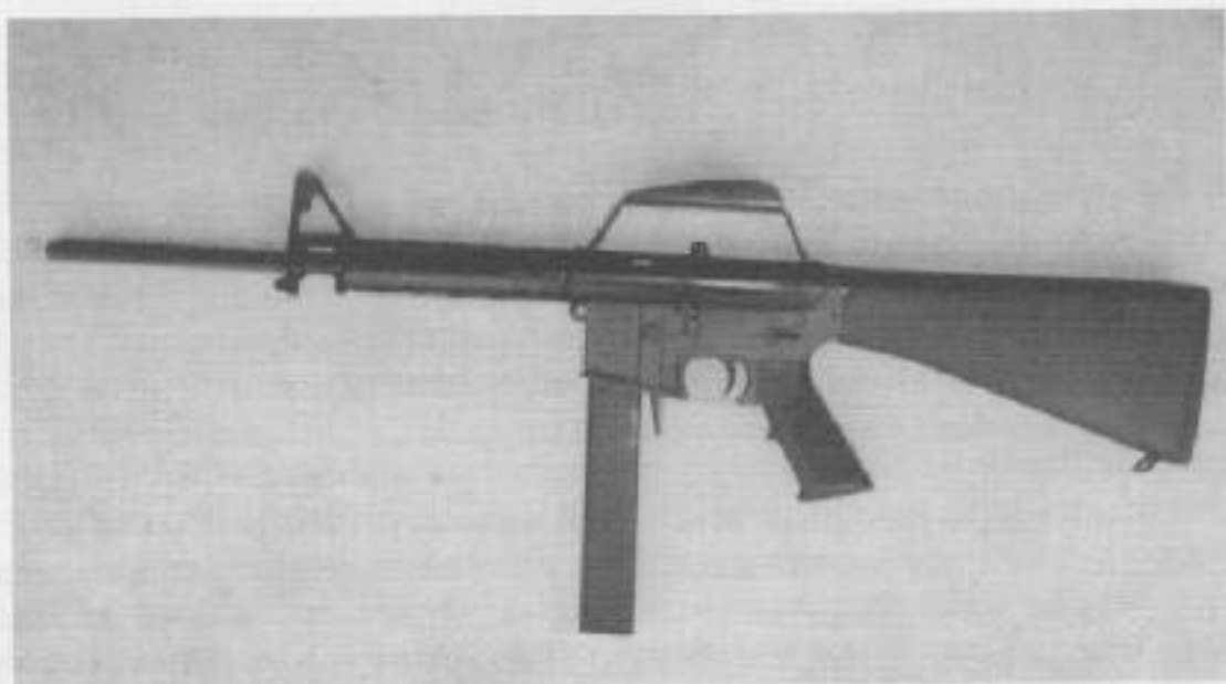
Full-length view showing unit mounted on Colt-made lower.
