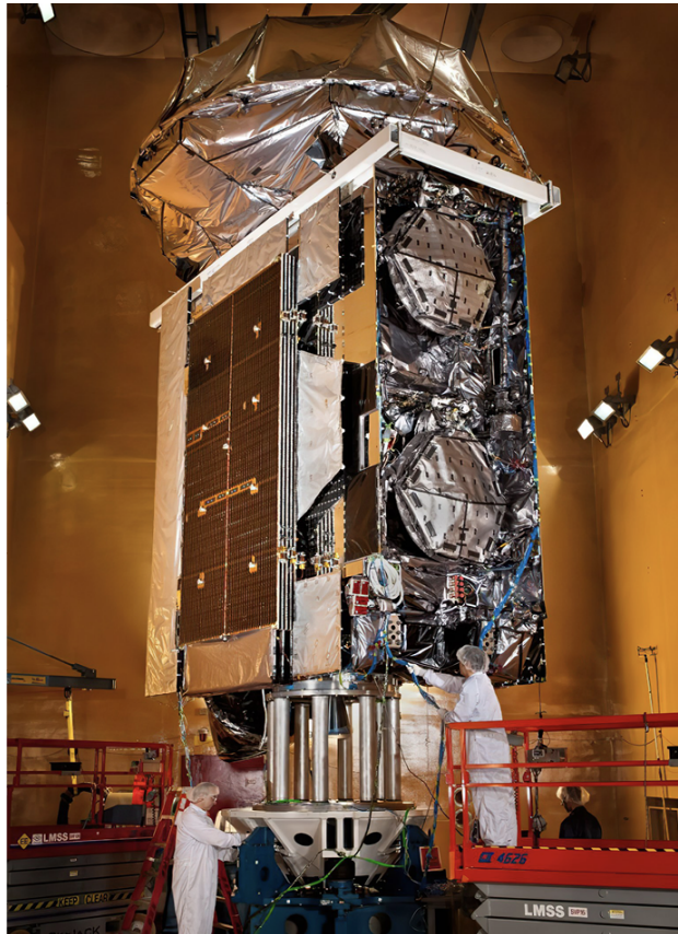
MUOS satellite (Mobile User Objective System). Ultra-high frequency (UHF) SATCOM system of four orbiting satellites and four relay ground stations (Space Fence). Developed by Lockheed Martin for the U.S. Navy. Note the hexagons. Reminds me of the film The Wicker Man (1973, 2006).
