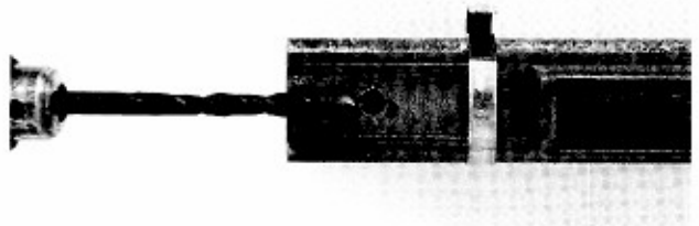
PHOTO 7: Drill through lower receiver bolt holes and into upper receiver tube.
