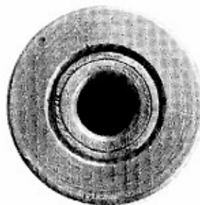
PHOTO 18: Breech view of barrel. Note bevel around mouth of chamber.
