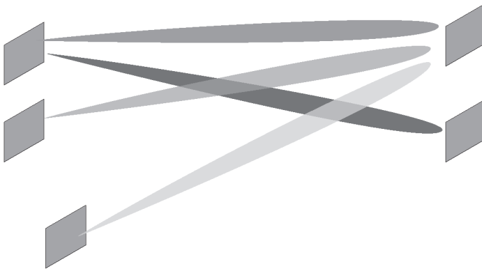
Figure 3.1 Spatial multiplexing using sharp beams is common at optical frequencies, and also possible at radio frequency (RF) and mm-wave frequencies using arrays or large apertures relative to the wavelength.
