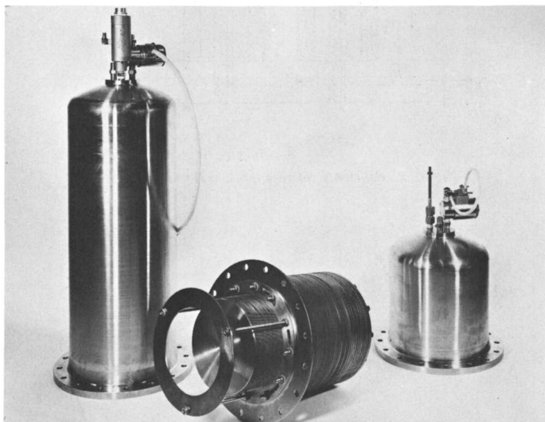
Figure 5. 500-Watt regenerative, hydrogen-oxygen, fuel-cell assembly
