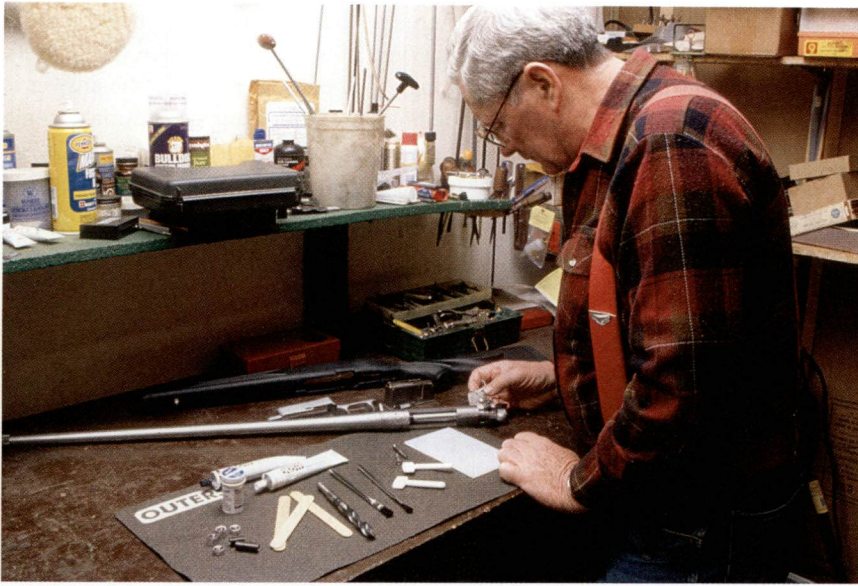
John R. Kascenska disassembles a rifle in preparation to pillar bed the stock. Here, he is inspecting the trigger.
