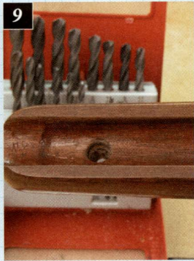
8. This shows a rifle stock clamped in a vise in a drill press in preparation for drilling. 9. Proper drill size is important to a quality installation of a sling swivel.
