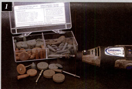
1. Dremel hand grinder with assorted Cratex polishing tools from Brownells. 2. Polishing and grinding tip kits from Brownells for use with Dremel type hand grinders.
