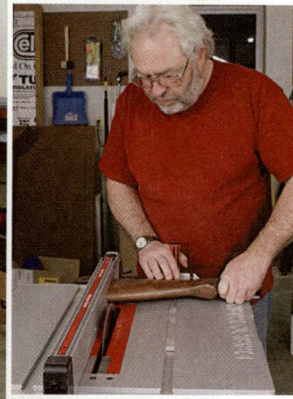
Author Bryce Towsley, in his shop (shown at right) cutting a stock off using a table saw.
