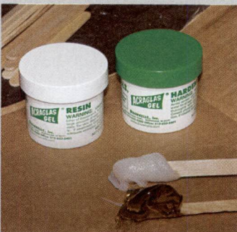
Acraglas Gel with dyes, thinner atomized metal and release.
