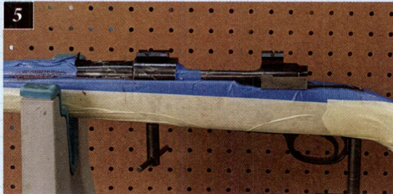
5. The assembled rifle with bedding compound. Shows the bedding compound oozing out around edges.
