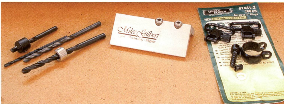
Tools and materials for installing sling swivels on a pump action rifle. Drills, alignment tool and swivels.
