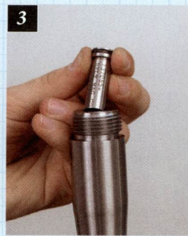
3. Inserting the "go" gauge into the chamber to check for the head-spacing.
