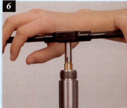
6. Reaming the chamber with a Clymer T-handle.
