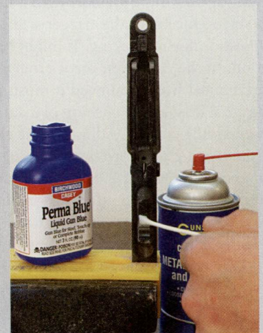
Rebluing the trigger guard with cold blue after the space is enlarged.
