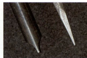
Tapered standard screwdriver on right and parallel straight side gunsmith's screwdriver on left.
