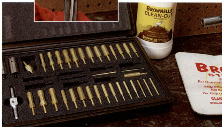
Brownells Chamfering & Facing Combo Set with pilots and cutters for crowning and facing barrels.
