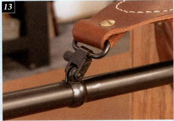
13. A completed installation of Michael's of Oregon band type sling swivel on a Remington 7600 pump-action rifle.
