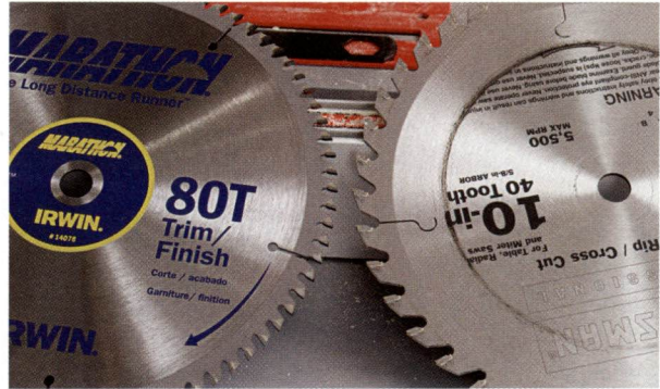
Top: For the best cut on a gunstock, use a carbide 80 tooth saw blade.
