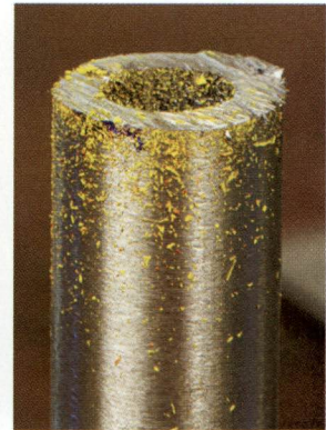
End of a rifle barrel after cutting it off with a hacksaw. Note below how it is uneven.
