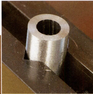
Rifle barrel muzzle after facing it off with a Brownells' 90-degree muzzle facing cutter.
