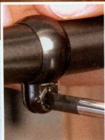
12. Installing the tension screw for a Michael's of Oregon band type sling swivel on a Remington 7600 pump-action rifle.
