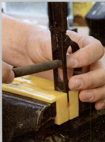
Using a file to open the space in the trigger guard on a Mini-Mauser to allow for a wider trigger.
