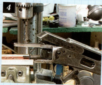
4. Drilling the new hole.
