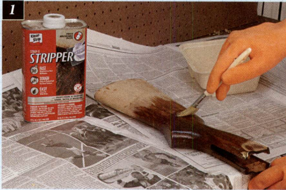
Stripping the old finish off a stock.
