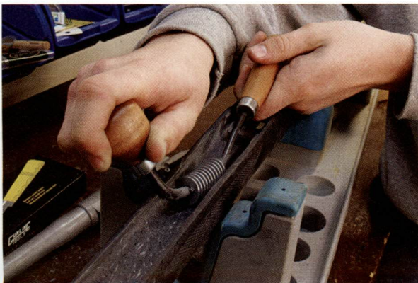
Brownells' Barrel Bedding Tool is used to scrape away material and open the barrel channel in a rifle stock.
