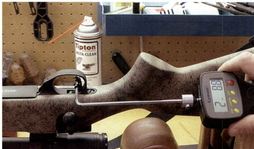
Installing a Timney trigger on this Weatherby Vanguard rifle has greatly improved the trigger pull.
