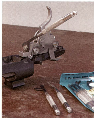
Adjusting the trigger on .458 Winchester Mauser. Wrenches are from Brownells.
