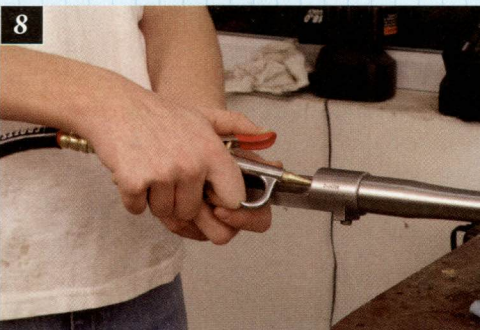
8. Cleaning the chips from the chamber with shop air before inserting the "go" gauge into the chamber to check for the headspacing.
