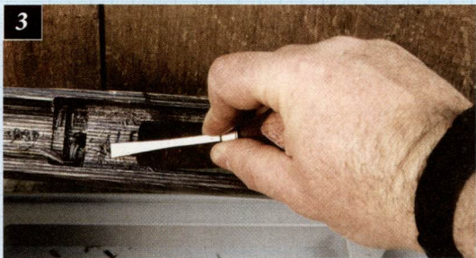
3. When removing wood from the action area in preparation for glass bedding, be sure to leave a section for support.
