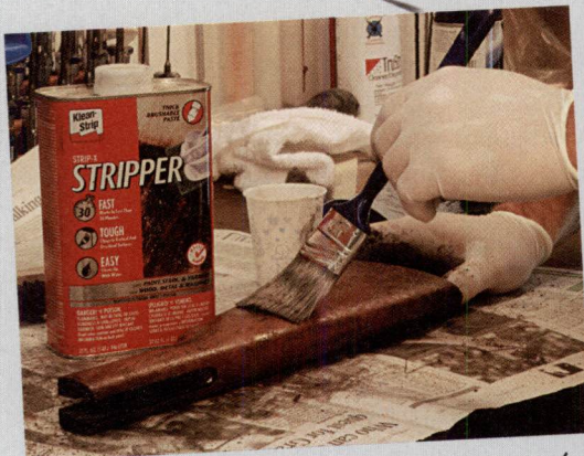
Stripping the old finish off a stock.
