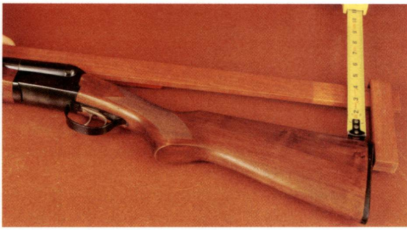
Measuring the drop on a shotgun stock with a Brownells Pull & Drop Gauge prior to installing a recoil pad.
