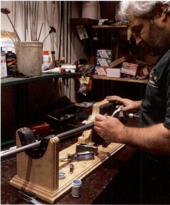
Above: Applying release agent to rifle metal.
