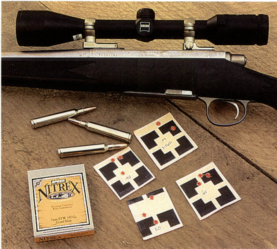
Remington M-700 BDL SS DM in 7mm STW. Zeiss Diavari 5-15 T* scope. With Nitrex 145-grain ammo. Shows the accuracy of the rifle after pillar bedding the stock and filling the barrel channel with Bondo.
