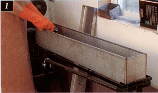
1. Final degreasing in preparation for DuraCoat. This tank contains TruStrip degreaser from DuraCoat.
