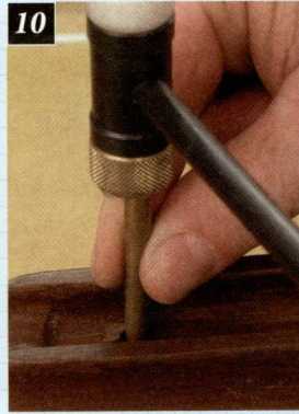
10. Using a brass punch to tap the knurled nut into place for installing a sling swivel stud on the forend of a bolt-action rifle. 11. All exposed wood should be coated with stock finish.
