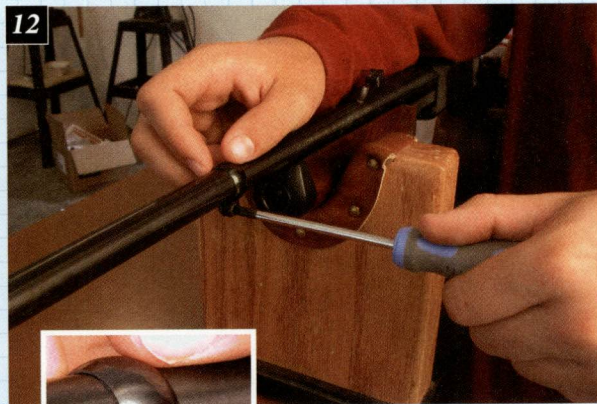
12. Installing the tension screw for a Michael's of Oregon band type sling swivel on a Remington 7600 pump-action rifle.
