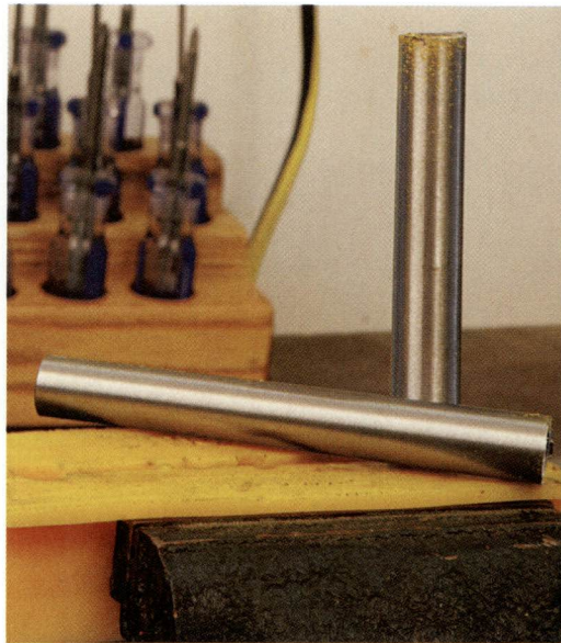
End of a rifle barrel after cutting it off with a hacksaw. Note below how it is uneven.
