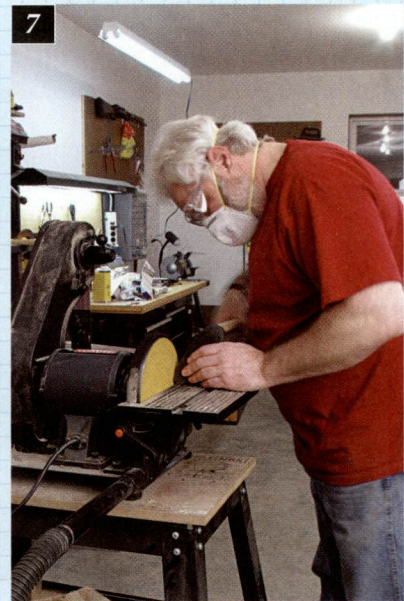
7. Shaping a recoil pad on a disk and belt sander. Note safety glasses and mask.
