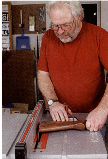
Top: For the best cut on a gunstock, use a carbide 80 tooth saw blade.
