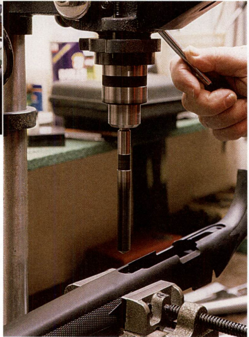
Below: Preparing to drill synthetic stock for pillar bedding.
