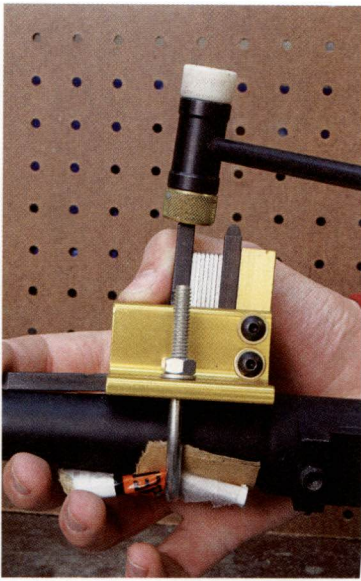
Stamping the numbers on the barrel, using Wheeler Engineering stamps and a B-Square guide sold by Brownells.
