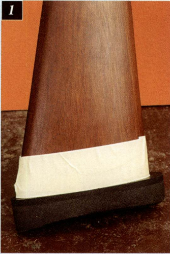
1. Masking tape wrapped on the stock to protect the finish while sanding the recoil pad. 2. Scribing a line on the recoil pad along the edge of the stock to allow sanding the pad on a jig.
