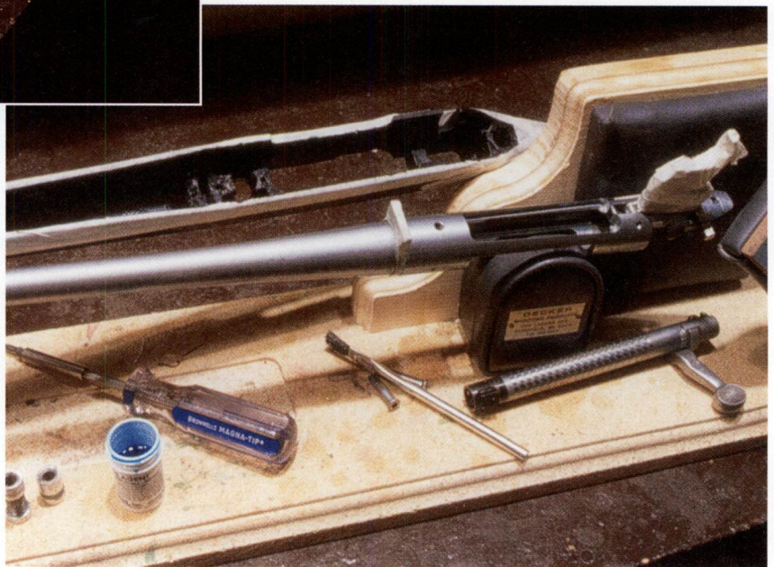
Above: Applying release agent to rifle metal.
