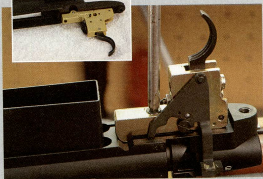
Installing a Timney trigger on a Weatherby rifle.
