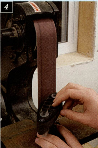
4. Sanding a recoil pad in Miles & Gilbert recoil pad sanding jig. 5. Shaping a recoil pad attached to the stock. 6. If the stock is going to be refinished, the best fit is by sanding the recoil pad and the stock at the same time.
