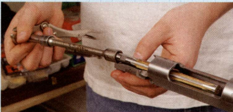
5. Reaming the chamber on a .458 Winchester barrel. Note the barrel in the action and the socket wrench extension with vise grips to turn it.
