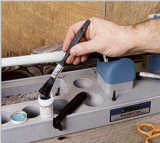
Painting release agent on barreled action before glass bedding. Note tape on barrel to create gap for floating barrel.
