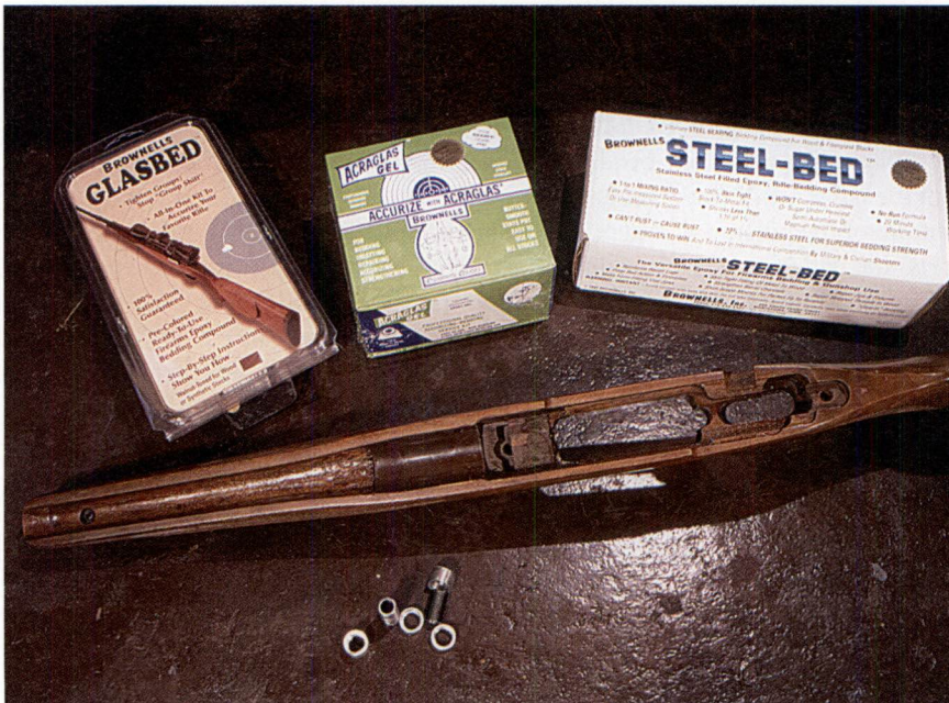
While this wood stock has been glass bedded without pillars, a variety of pillar kits are available on the market.
