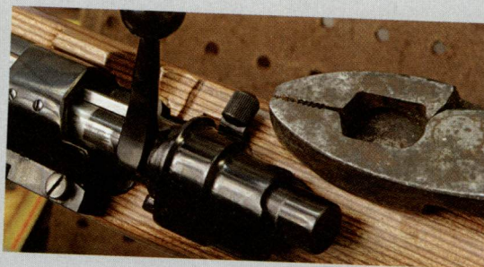
Using pliers to bend the safety on a Timney trigger so it will clear the bolt on a Mini-Mausser rifle.
