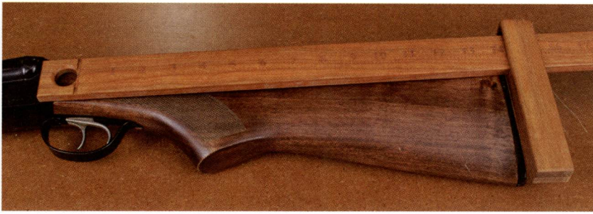
Measuring the length of pull on a shotgun stock with a Brownells Pull & Drop Gauge prior to installing a recoil pad.
