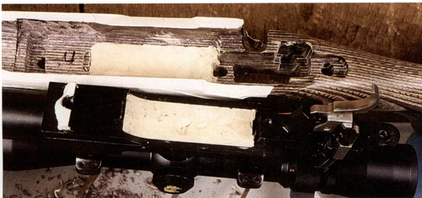
Rifle action and stock with clay filling the action and magazine opening to keep bedding compound out. Stock has masking tape to protect against overflow of bedding compound.
