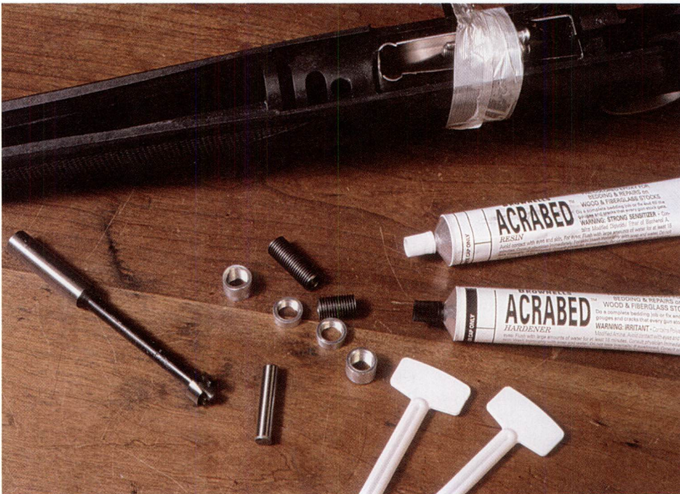
Remington synthetic stock, Brownells Acrabed, pillars and pilot drill. Note the removable pilot on the drill.
