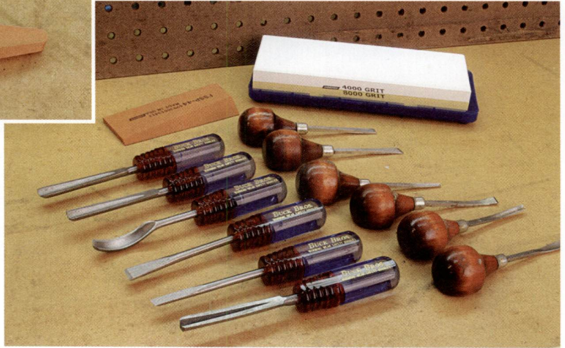
A set of wood carving hand chisels. Shown with a Norton India slip stone, and a larger Norton water stone.
