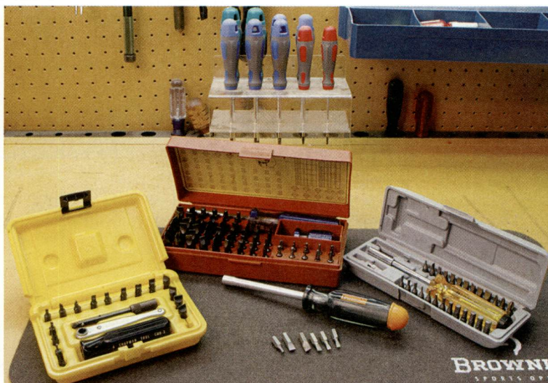
Working on guns will require specialized screwdrivers. There are kits available from a lot of different suppliers. These are from Chapman, Brownells, Midway and Lyman.
