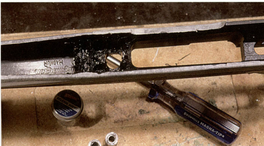
Shows the Remington M-700 BDL SS DM stock. Note that the area around the action has been roughed up and anchor holes have been drilled for bedding material. Hole for pillar is drilled and masking tape is applied.
