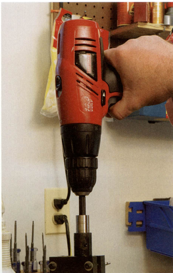
Left: Brownells 79° crown cutter being used in drill to add a radius to the outside of the barrel's muzzle. The finished muzzle is shown above.
