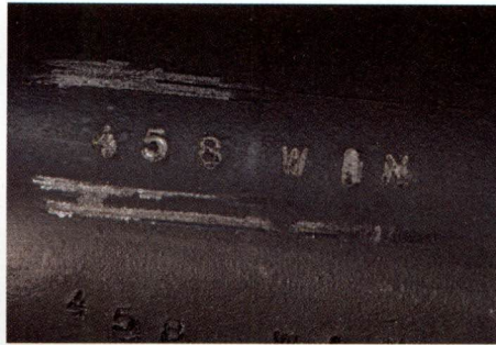
Stamping the numbers on the barrel, using Wheeler Engineering stamps and a B-Square guide sold by Brownells.
