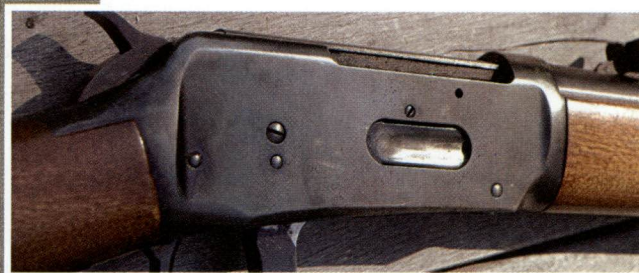
Note the rust on receiver around the loading gate.
