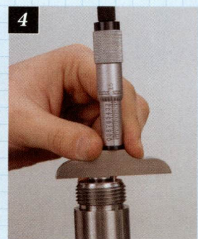
4. Measuring from the back of the "go" gauge to the face of the barrel.
