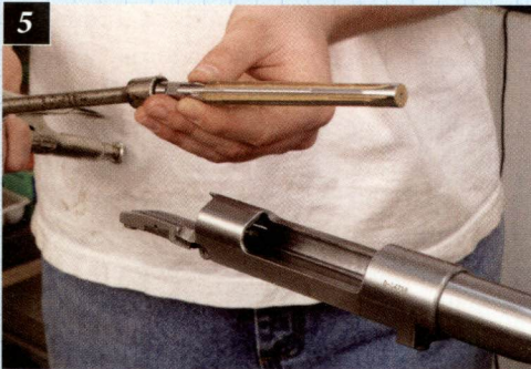
1. Using a depth micrometer to measure from the front of the action to the bolt face.
