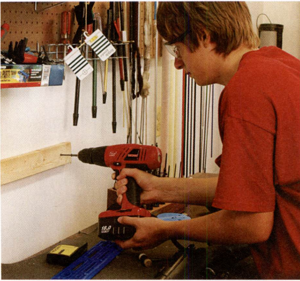
Nathan Towsley uses a cordless electric drill to install shelf brackets over the workbench.
