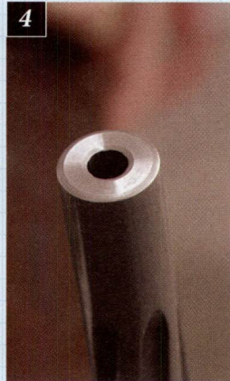
4. This rifle muzzle has been faced off with the Brownells Muzzle Facing Tool and then re-crowned with a 45-degree cutter.
