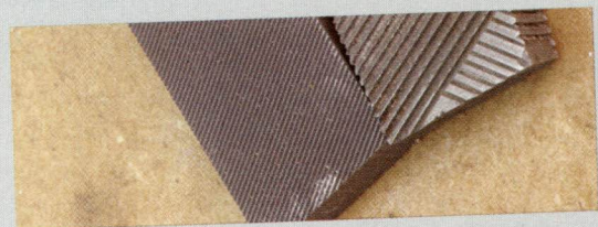
Mill or single cut (left) and double cut or flat file.
