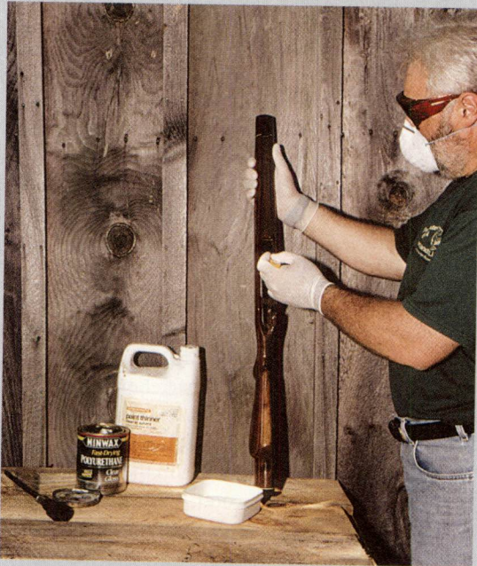
Applying thinned polyurethane.
