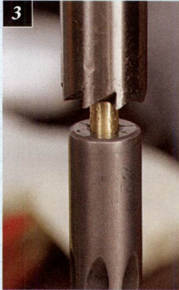
3. Shows the Brownells Muzzle Facing Tool in use. This tool cuts the face of the barrel square with the bore.
