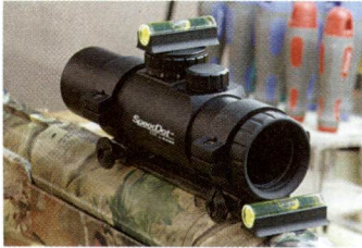
Using the Level-Level-Level to align an aimpoint red dot sight.
