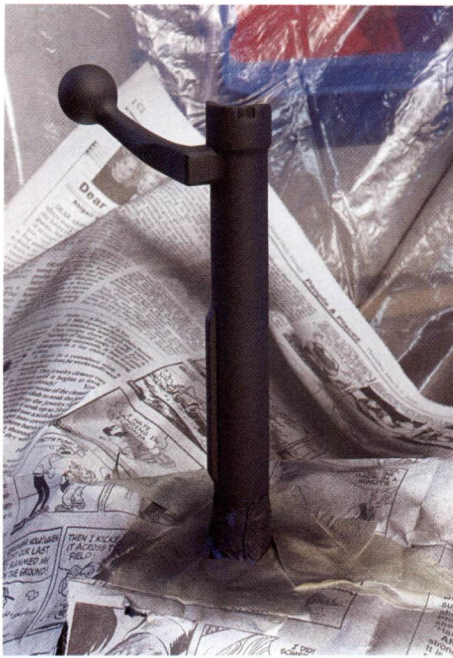
The Mauser bolt after applying DuraCoat finish.
