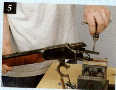
5. Tapping the new hole.
