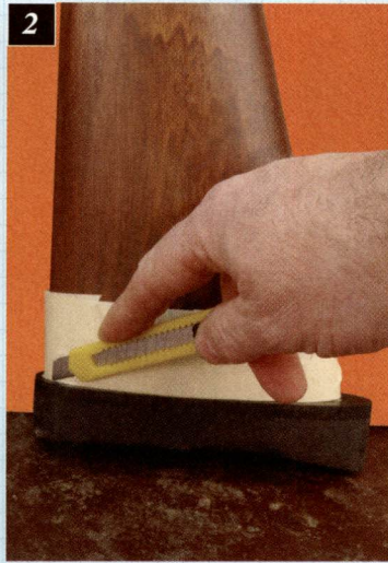
1. Masking tape wrapped on the stock to protect the finish while sanding the recoil pad. 2. Scribing a line on the recoil pad along the edge of the stock to allow sanding the pad on a jig.
