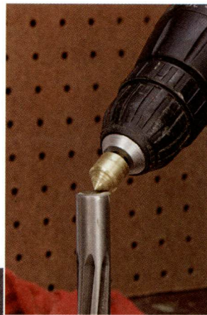
Brownells Chamfering & Facing Combo Set with pilots and cutters for crowning and facing barrels.
