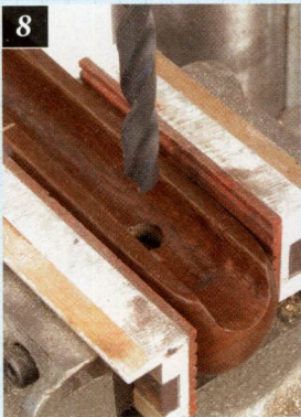
8. This shows a rifle stock clamped in a vise in a drill press in preparation for drilling. 9. Proper drill size is important to a quality installation of a sling swivel.
