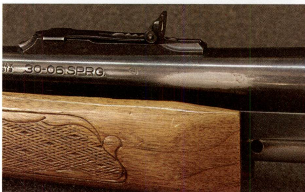
Two examples of oval patches where the bluing has worn off of this Remington 760, due to abrasive leather gloves.
