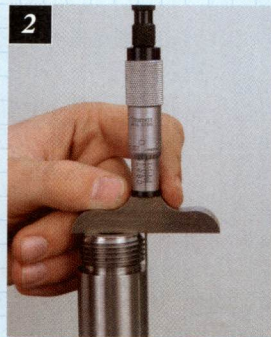
2. Measuring the length of the barrel shank.
