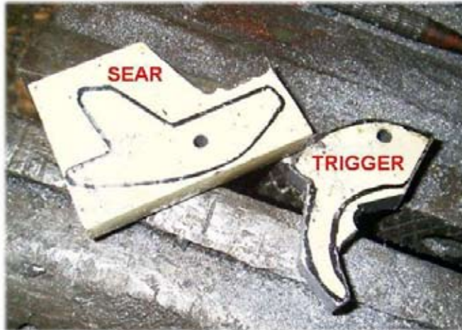
These parts are made from 10mm thick steel
