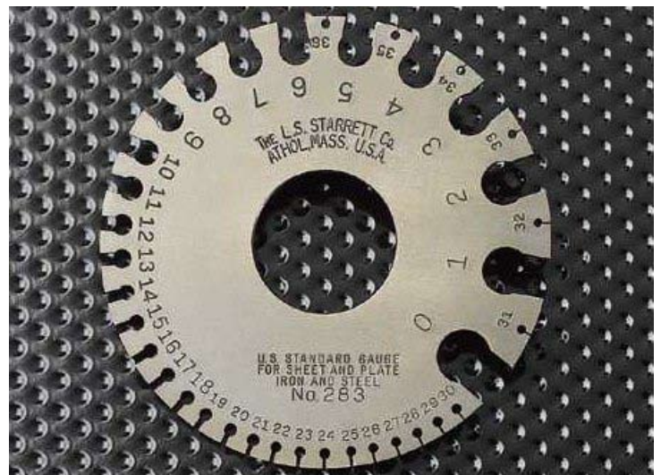
The picture above illustrates how to use a sheet metal gauge. You just slip the sheet metal into the gauge, and the thickness, or gauge, can be quickly determined. Starrett gauge is below.
