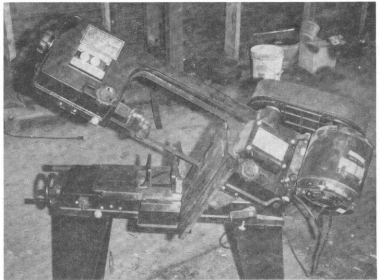
Below: A small metal cutting band saw such as this can save a lot of manual labor.
