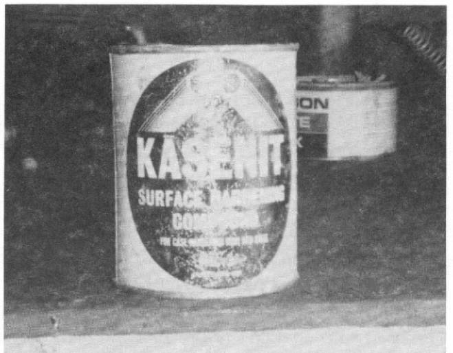
Low-carbon steel can be hardened using compounds such as Kasenit, as shown. Several other similar compounds are also available.
