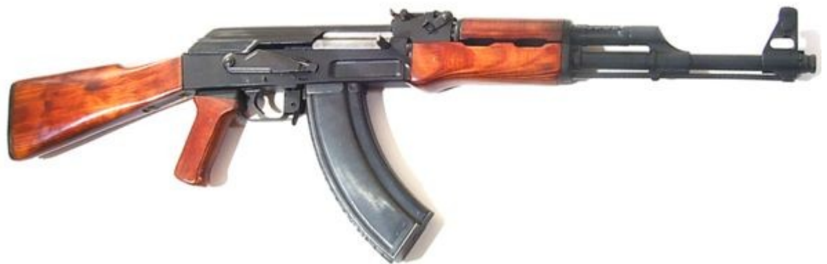
Modified AK (1955 manufacture), with machined receiver. Note the distinctive machined cuts above and forward of the magazine well.
