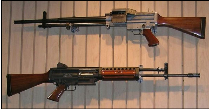
7.62mm Stoner 62 weapons in light machine gun (top) and rifle (bottom) configurations
