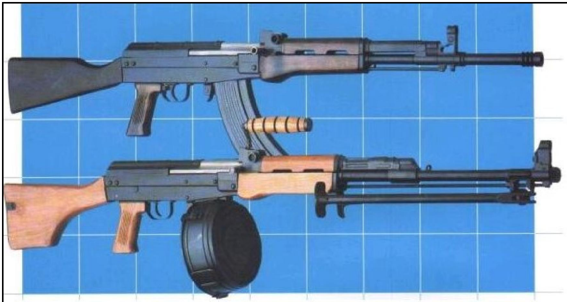
Type 81S (late production export version with fixed butt) assault rifle (top) and Type 81MGS light machine gun (bottom)
