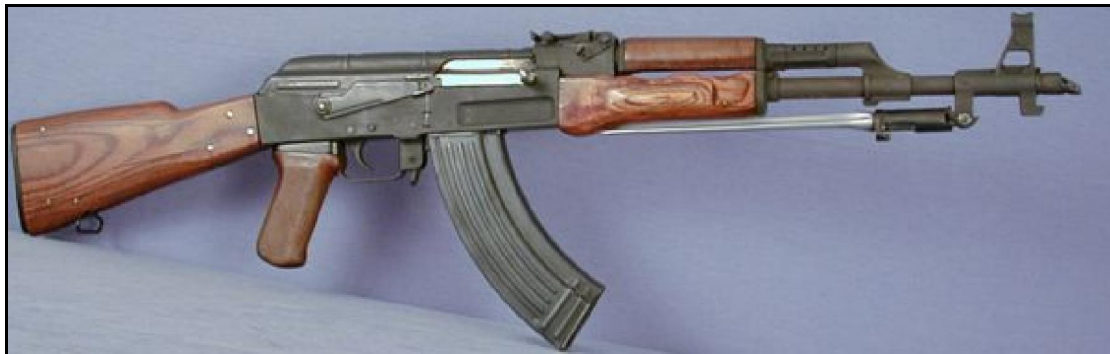
Type 56 assault rifle with machined (milled) receiver
