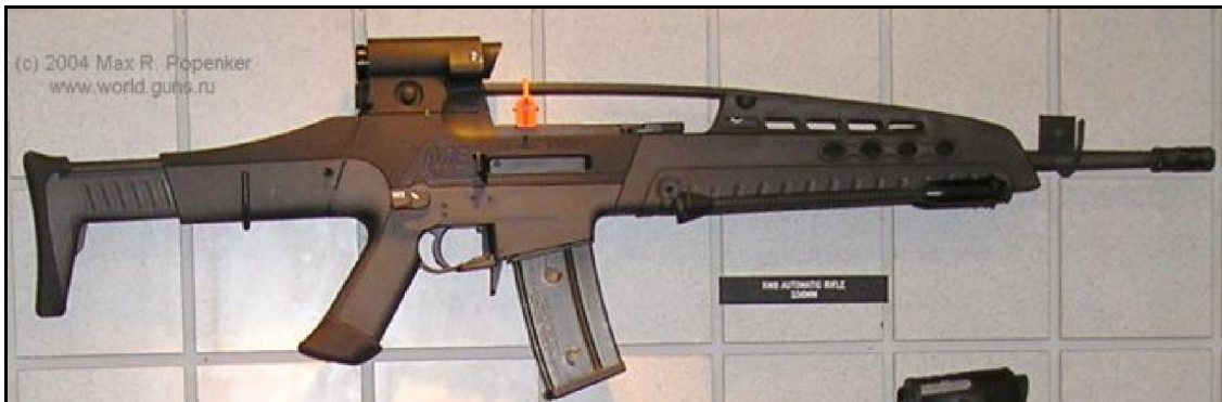
XM8 rifle in "automatic rifle" (light machine gun) configuration. Note longer barrel and folded bipods under the forearm
