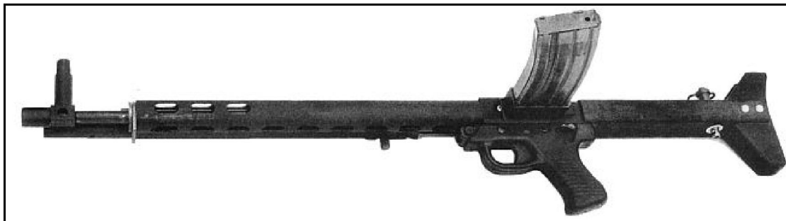
TRW LMR (Low Maintenance Rifle) in its final shape, left side, with 30-round magazine attached
