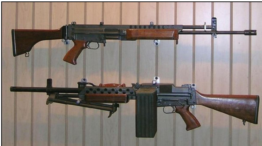
5.56mm Stoner 63 weapons, in rifle (top) and light machine gun configurations
