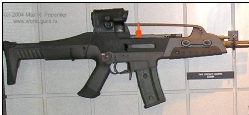
XM8 rifle in Compact (SMG / PDW) configuration, with shortened barrel
