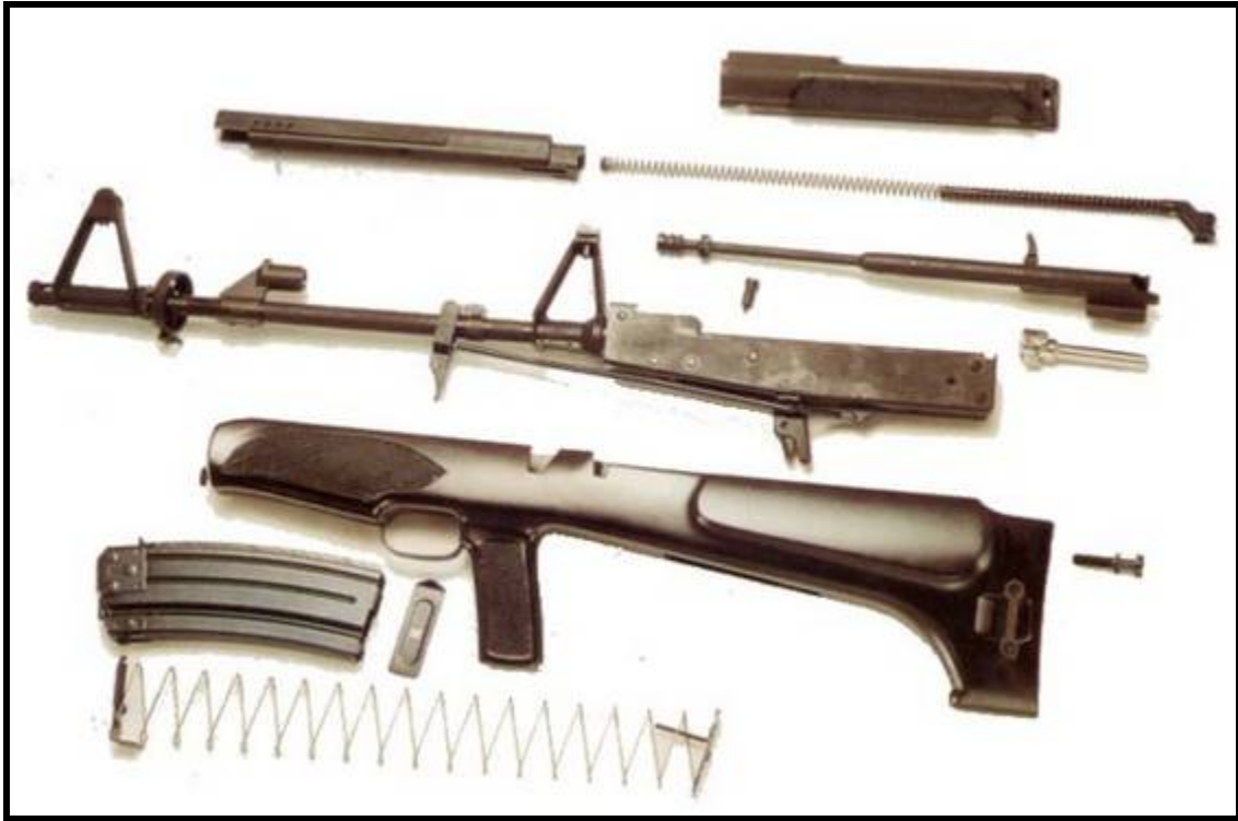
Valmet Model 82 rifle, partially disassembled
