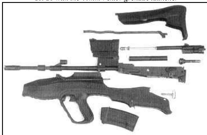
CR-21 disassembled into major components
