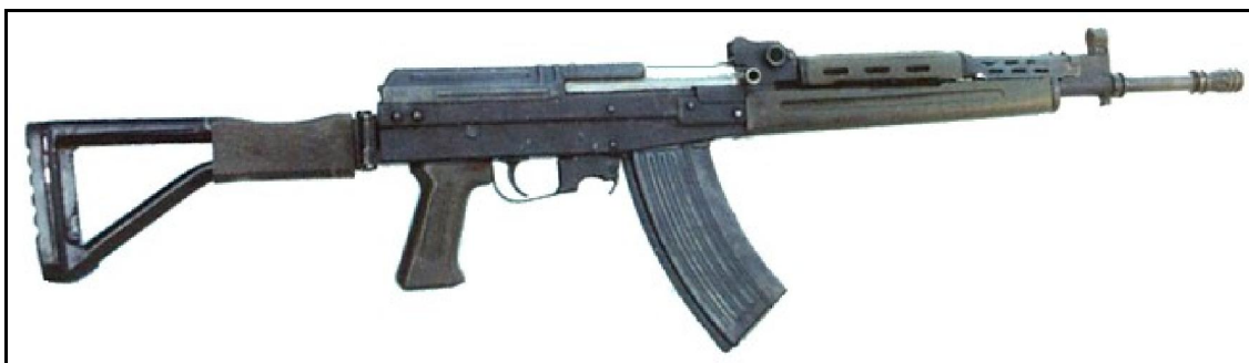
5.8x42 Type 87-1 experimental assault rifle, used to develop and test 5.8mm DBP87 cartridge for QBZ-95 rifle
