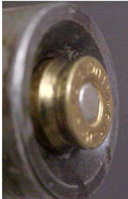
Original STEN chamber feed entrance:
