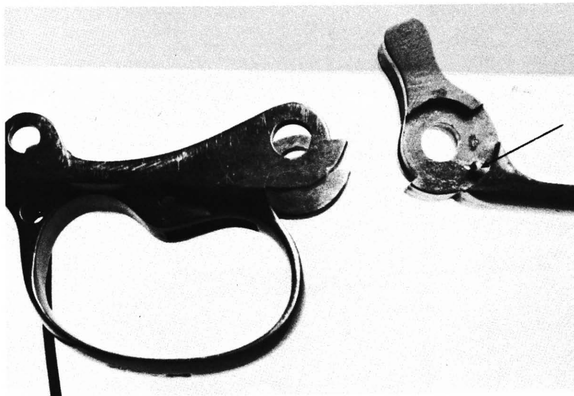
Fig. 3-17. Arrow points to the spring-backed plunger in a hole drilled into the Martini finger lever to provide tension to hold the lever closed. The trigger guard is notched at the spot at the end of the plunger's travel when the action is closed.
