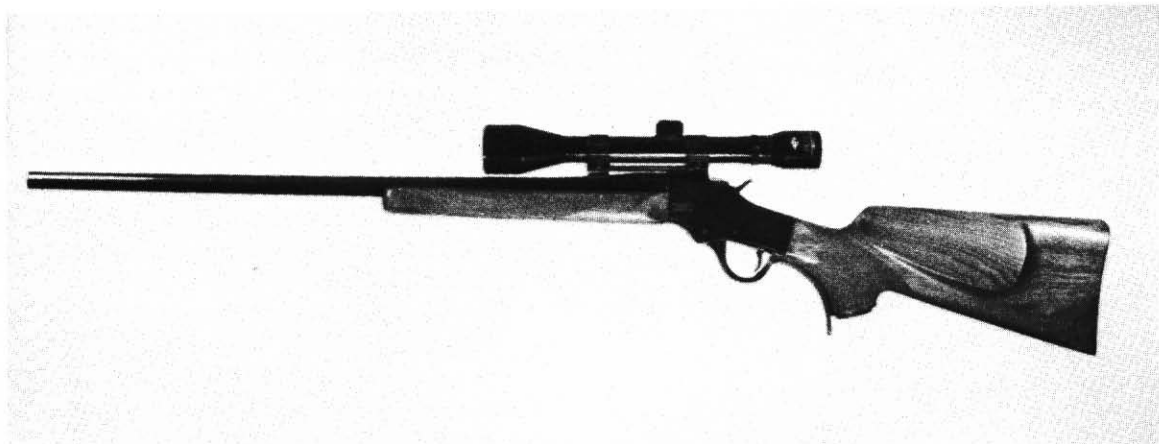
Fig. 4-5. My eight-pound varmint/deer rifle in .243 caliber was built on the FBW Model S action. It is fitted with a 25" Shilen sporter barrel and a Fajen stock and forearm. The 6× scope is mounted in Weaver top detachable rings on a Weaver No. 50 one-piece base.
