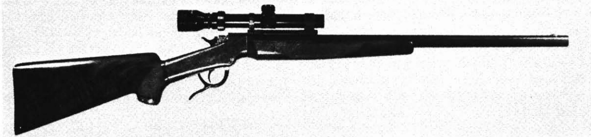
Fig. 12-5. My custom Marlin Ballard .22 LR small game rifle; the 2.5—5 \times Tasco scope is mounted with a Redfield Jr. mount having a flat bottomed base to fit an octagonal barrel. A Redfield Jr. base made for the Remington Model 760 rifle could have been used, with or without flattening the bottom of the base. The base could also have been mounted part on the receiver top and part on the barrel and this might have been necessary had a different scope been used—a hunting scope with an enlarged objective end, for example.
