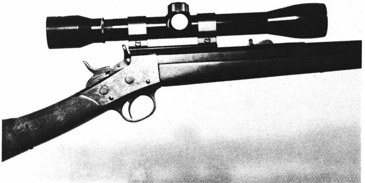
Fig. 2-2. A Remington No. 2 rifle originally in .22 rimfire caliber restored to shooting condition by reboring and rechambering the barrel to .25-20 W.C.F. The scope is mounted with Weaver tip-off rings and a tip-off base for the Marlin Model 39A.
