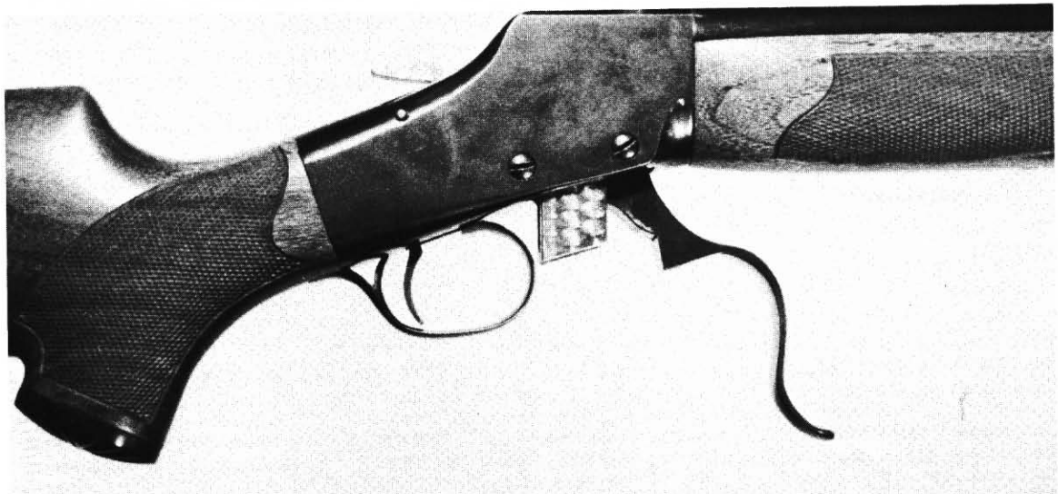
Fig. 4-26. The action open on the Model J with the altered trigger guard and finger lever.
