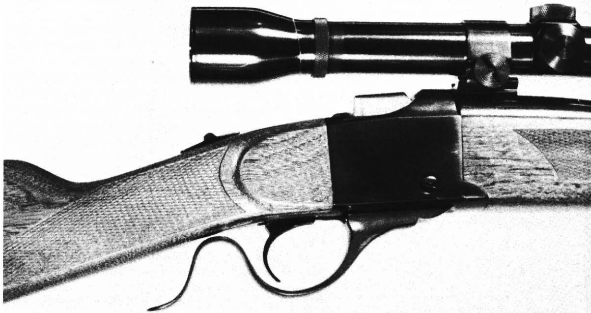
Fig. 7-5. Close-up of the finished grip panels. This remodeled grip greatly enhances the looks and the feel of the rifle.
