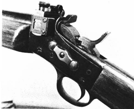
Fig. 2-25. A receiver sight made for the Model 70 Winchester is readily adaptable for mounting on a large rolling block action.
