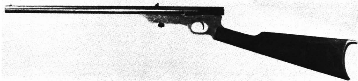
Fig. 10-5. This long-obsolete Quackenbush boy's .22 rimfire rifle is worthy of a complete restoration—rebluing the barrel, renickeling the frame, color case-hardening the breechblock, and refinishing the stock.
