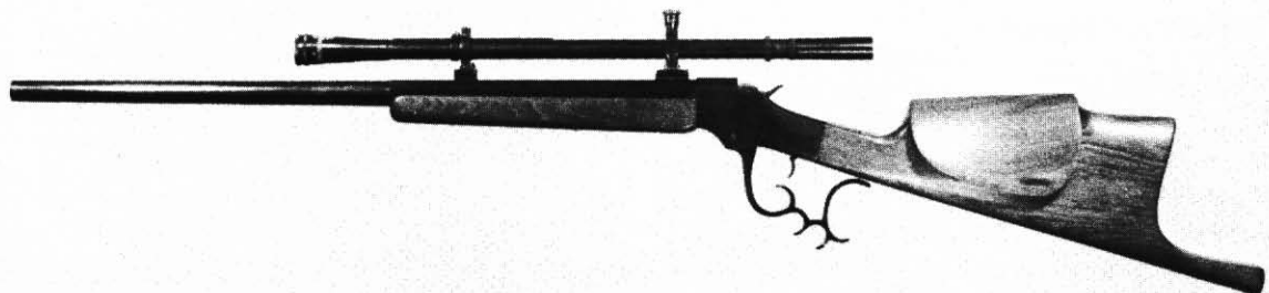
Fig. 4-6. My Schuetzen-styled target rifle is built on the Model S action with the Schuetzen finger lever. The half-octagon barrel is tapered from 1.20" across the flats at the breech to .800" at the round muzzle and is topped with a Lyman Jr. TargetSpot scope. A novel feature of the buttstock is the integral wood prong, made so to avoid the necessity of purchasing or making a pronged butt plate. This rifle is chambered for the .30-30 cartridge, and it has proven extremely accurate. Weight without scope is ten pounds.
