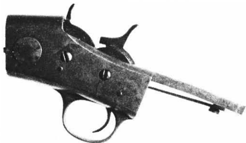
Fig. 2-6. The Crescent rimfire rolling block action. It was used for rimfire cartridges only and is a close copy of the No. 4 Remington.
