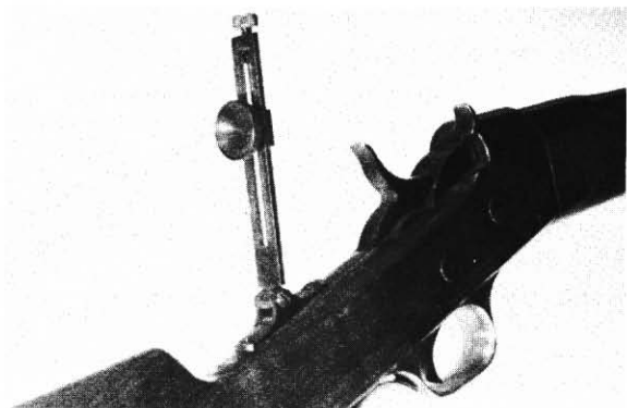
Fig. 9-4. This long-range tang aperture sight obtained from Navy Arms is a replica of a sight used long ago on target rifles such as the one described here.
