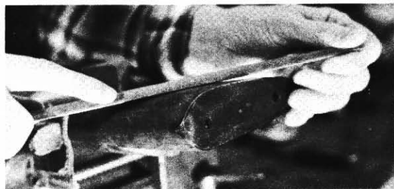
Fig. 5-4. Wood rasps are used to trim off excess wood from the stock and forearm.
