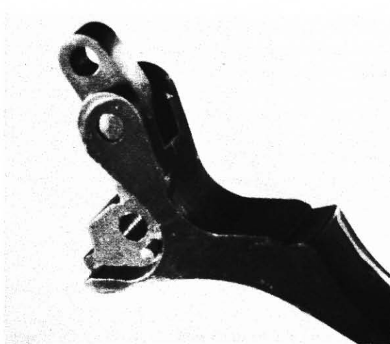
Fig. 4-16. This close-up photo shows the location of the spring-backed plunger in the Model L finger lever base to provide lateral tension to the extractor when altering it to handle a rimless or belted cartridge.
