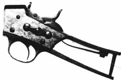
Fig. 2-7. A refinished and color case-hardened No. 2 Remington action, my favorite.
