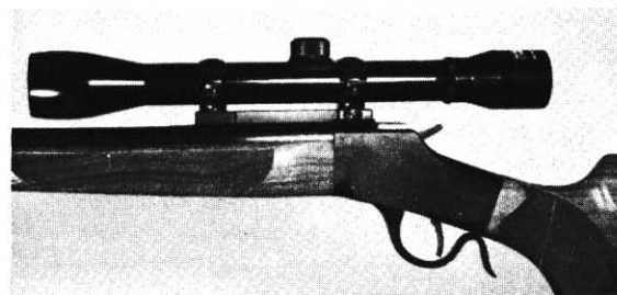
Fig. 4-30. Close-up of the FBW Model K rifle showing the Redfield Jr. scope mount. The base of this mount is one made for the Rem. M-760. The rear end of this base was machined flat to fit the receiver ring and the base attached to the barrel and receiver with three screws.
