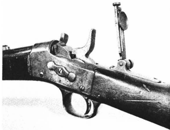
Fig. 2-26. A reproduction of the early vernier tang sight for use on many old single shot rifles is presently available and can be used on the large Remington, Whitney and other rolling block actions. See also pages 160-165.
