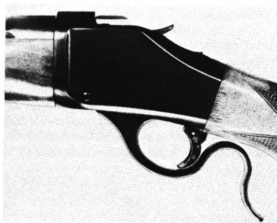
Fig. 8-4. As factory issued the Browning M-78 trigger has considerable slack or takeup and overtravel and there are no adjustments provided to eliminate this excess trigger movement. The weight of pull adjustment is also very limited. The best way to improve this trigger is to replace it with the Canjar single-set trigger mechanism as shown here. With this trigger mechanism you have the choice of either an adjustable single stage trigger or a single-set trigger that is adjustable to a pull of only a few ounces. (Courtesy Canjar.)
