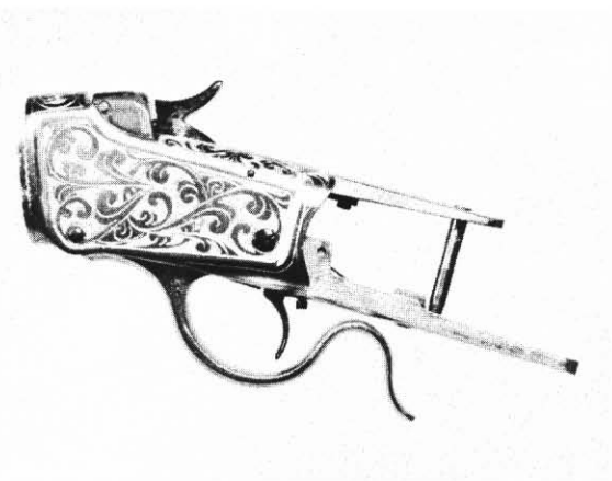
Fig. 1-21. This engraved early version low-wall action with the original S-shaped finger lever is ideal with a straight grip stock.
