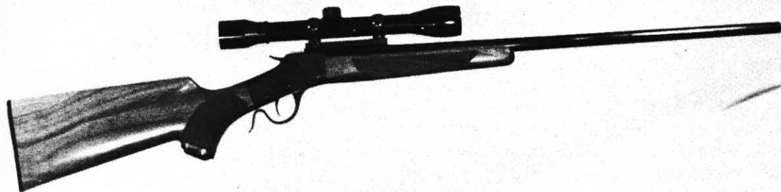
Fig. 4-2. The light varmint rifle that I built on the FBW Model K action. It is fitted with a 24" Federal sporter barrel in .222 Rimmed caliber. The 10× Universal scope is mounted in a Redfield Jr. mount. Although it weighs only 6.5 pounds the rifle is extremely accurate. The walnut stock is fitted with a horn buttplate and pistol grip cap.
