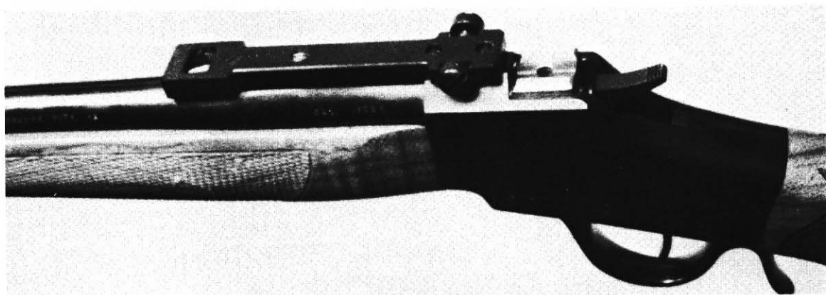
Fig. 12-3. Redfield Jr. scope mount bases made for a number of non-bolt action rifles which have the bridge in the center of the mount such as this one are adaptable for use on many single-shot rifles. The Redfield Jr. bases of this type include those made for the Remington Models 121, 241, 81, 141, 740, 742 and 760; Winchester Models 63, 61, 88, and 100; Marlin Models 39, 39A, 336, and others. On the FBW Model K actioned rifle shown here I used a base made for the Remington Model 760 and the only alteration it required was to machine or file the rear end of it flat underneath to fit the flat-topped receiver.
