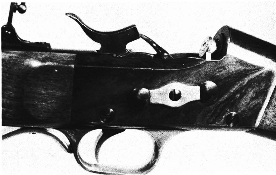
Fig. 9-3. Close-up of the opened rolling block action showing the extractor and a cartridge in the chamber.
