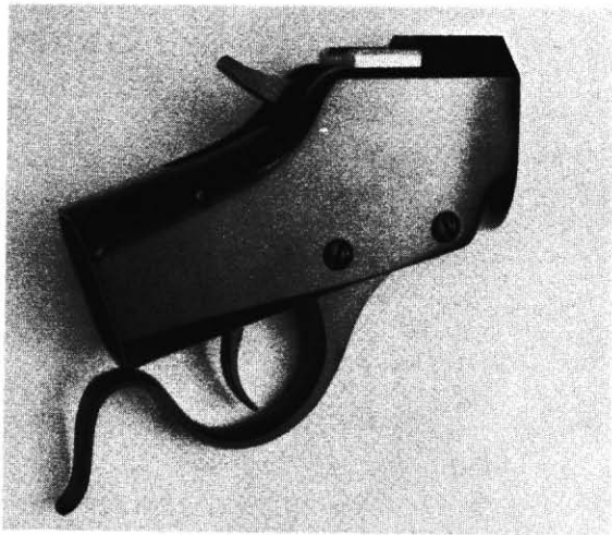
Fig. 4-7. The FBW Model J action. This is the standard or medium-sized FBW action suitable for most rimmed and rimless cartridges from .22 Hornet to .45-70 and from .222 to .30-06. Like all of the other FBW falling block actions, the Model J is of simple design and construction, with the major parts made by the investment casting process of the best steel, and heat treated.
