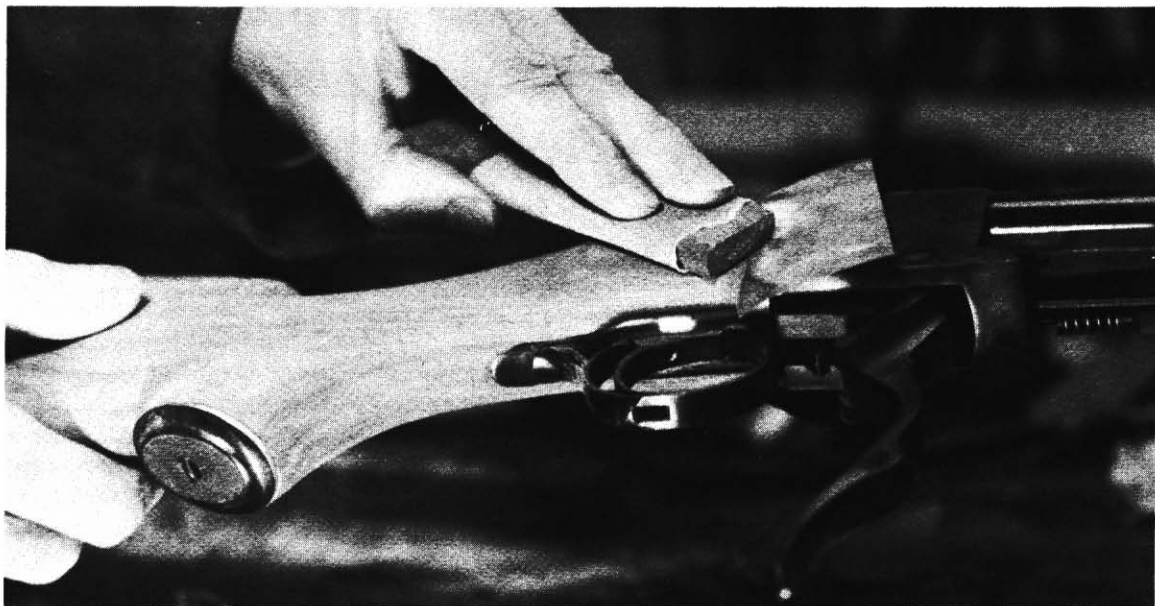
Fig. 5-5. To prevent scratching the blued finish of the receiver while sanding the grip panels, a piece of thin shim stock is placed between the stock and receiver.
