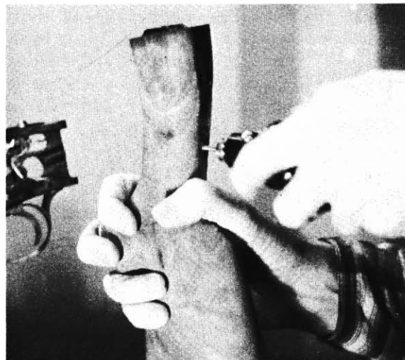
Fig. 5-2. A Dremel tool is used to remove small amounts of excess wood in some of the inletted areas.
