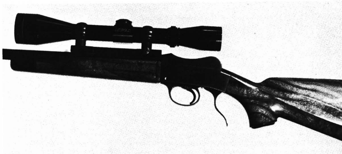
Fig. 3-6. Gunsmith H. L. Grisel worked out this finger lever design for the Martini Cadet action.
