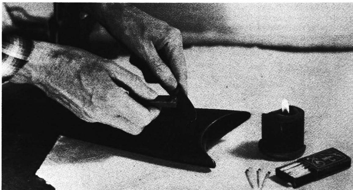
Fig. 10-7. Small cracks, holes and damaged spots in the stock wood can be hidden by filling with sealing wax stock filler stick. Glass-bedding compound dyed to match the wood can also be used.
