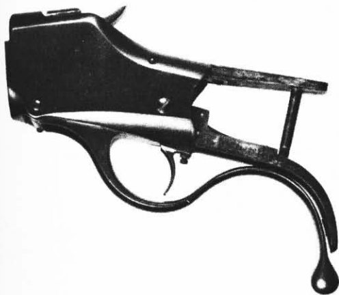
Fig. 1-18. A Neidner remodeled high-wall action, showing lower tang bent for a pistol grip.
