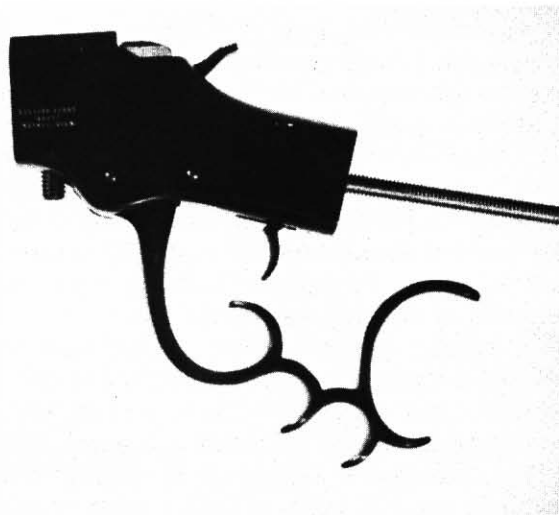
Fig. 4-3. The Model S action is shown here fitted with the Schuetzen-styled finger lever.
