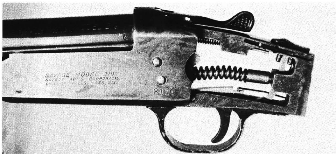
Fig. 11-4. The Model 219B Savage action with stock removed. The Models B, C, and L M-219 actions had inside swinging hammers rather than a striker as in the original Model 219.
