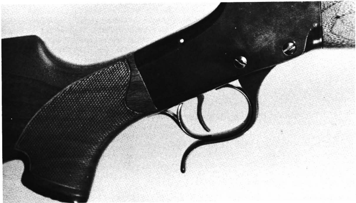
Fig. 4-25. Close-up of the trigger guard and finger lever remodeling on the Model J action showing action closed.
