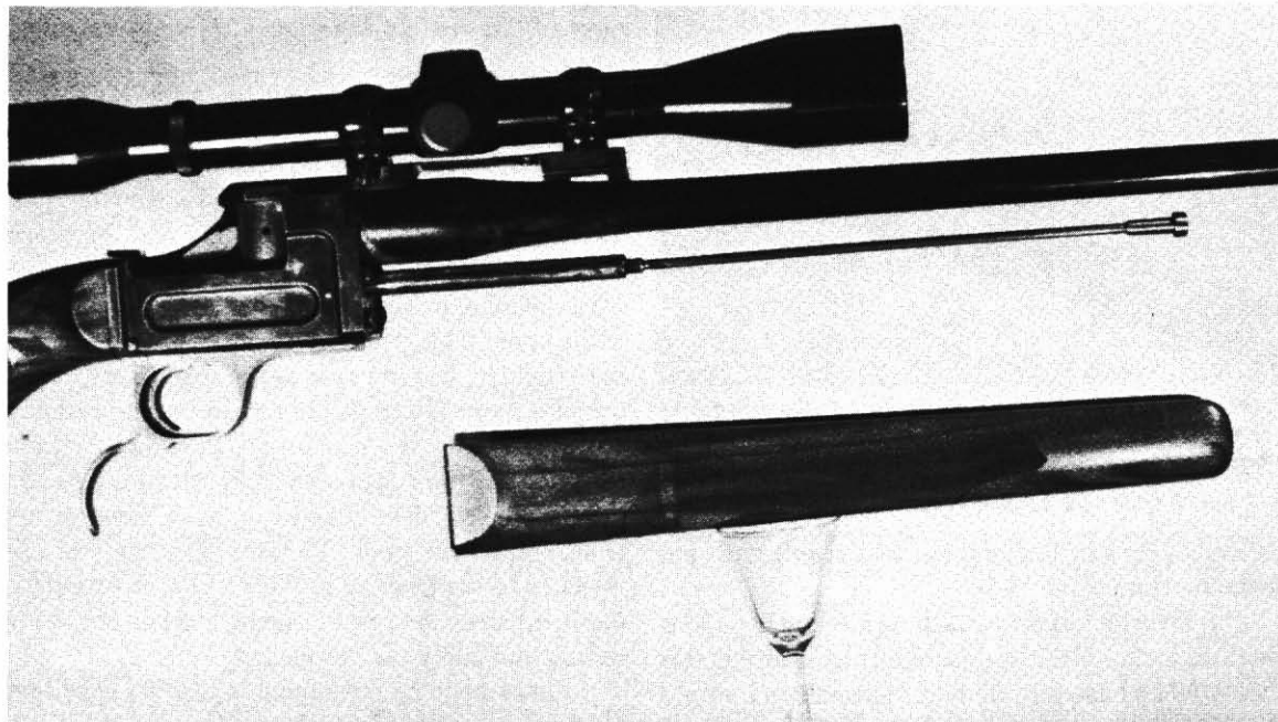
Fig. 12-9. Forearm removed from a rifle that is rigged up for a throughbolt forearm fastening method. The base of this fastening is attached to the receiver with four screws and the thin large-headed drawbolt threaded into it as it would if the forearm were in place. The base with its heavy rod does little to secure and support the forearm in the free-floating position; rather, the rigidity needed for this is obtained by perfect glass-bedded inletting of the forearm against the front of the receiver and a tight drawbolt to hold it there.
