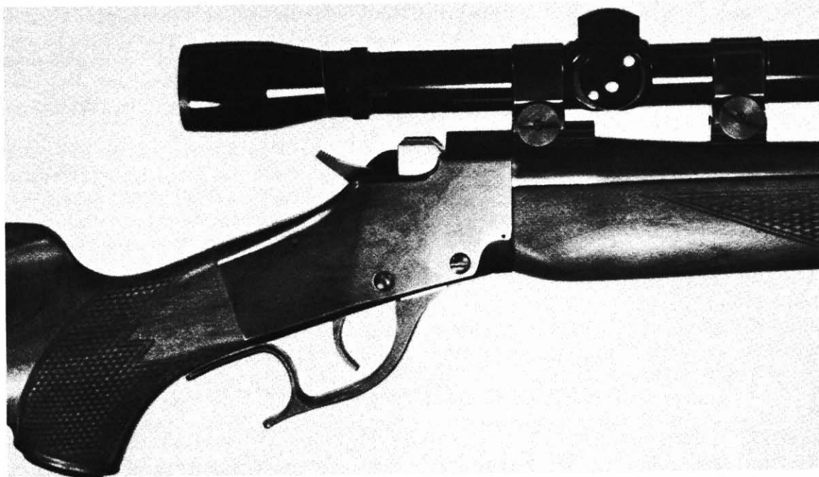
Fig. 4-20. A close-up view of the stocked FBW Model L action. The lowered right side receiver wall permits much easier access for loading and unloading and better access to the hammer. The altered finger lever provides more finger room and greatly reduces the chances of bruised fingers from firing the heavy-recoiling rifle.
