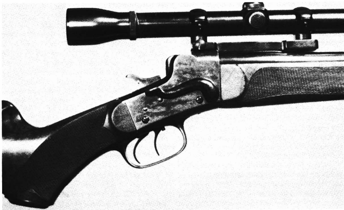
Fig. 12-4. A Redfield Jr. scope mount base made for the Remington Model 742 rifle was altered underneath to fit the barrel and receiver ring of this custom Remington-Hepburn varmint rifle. Three 6 \times 48 screws threaded into the barrel adequately hold the mount in place.
