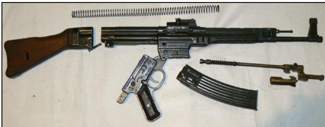
MP 43 assault rifle partially disassembled
