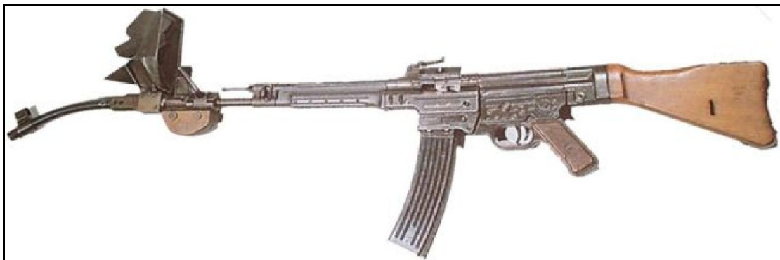
Stg.44 assault rifle with the Krummlauf Vorsatz J (curved barrel) attachment, which was designed to be fired "around the corner" or from inside the armored vehicle
