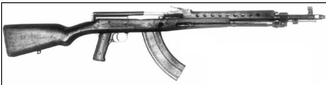
Tokarev 7.62x41 experimental assault rifle, as tested in late 1945
