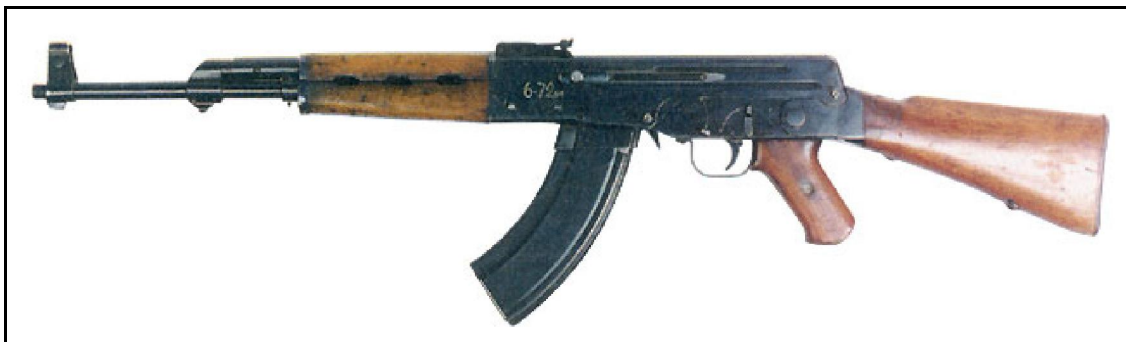
The first Kalashnikov assault rifle prototype of 1946, also known as AK-46. Note that it had numerous internal and external differences from the later models, including separate safety and fire mode selector switches, as well as non-reciprocating charging handle, all located on the left side of the weapon
