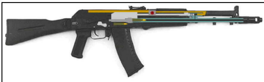
Illustration of the balanced action, with dual, counter-moving gas pistons above the barrel.
