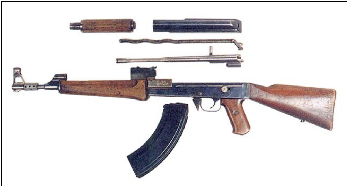
The experimental Kalashnikov assault rifle of 1947, also known as AK-47, first model, disassembled
