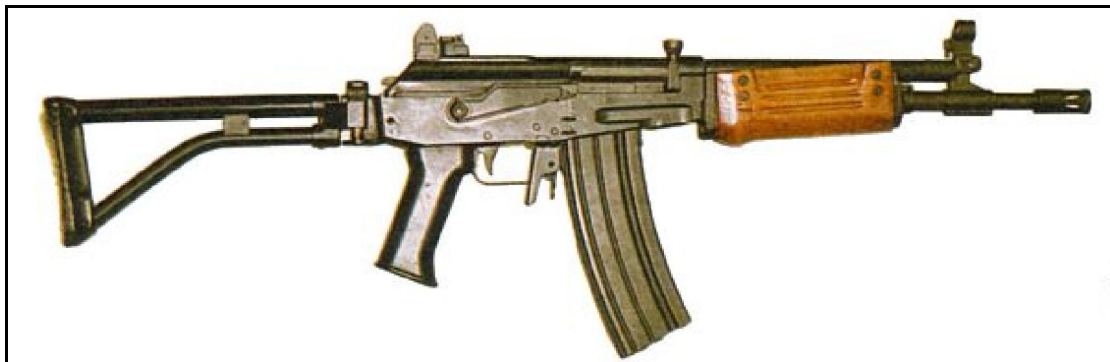
Galil SAR 5.56mm with shorter barrel (with older type brownish color wooden forearm)
