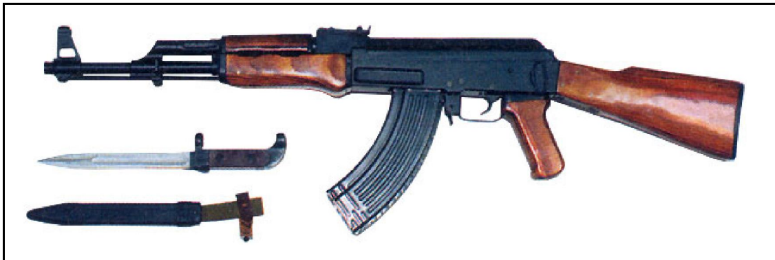
Post-1951 production Kalashnikov AK rifle with milled receiver and bayonet, left side
