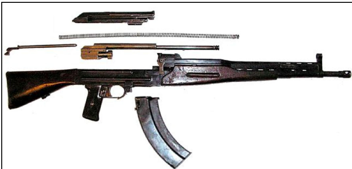
Bulkin AB-46 experimental assault rifle, partially disassembled.
