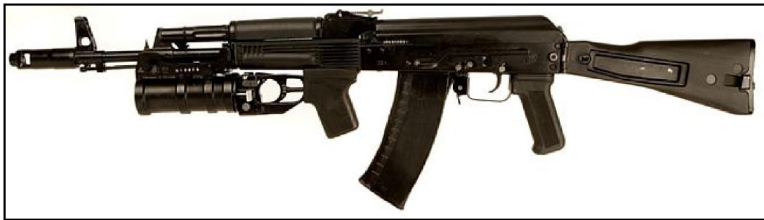
AK-74M with GP-30 40mm grenade launcher installed
