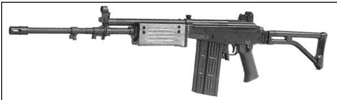
Galil AR 7.62mm. Note the longer barrel and deeper magazine
