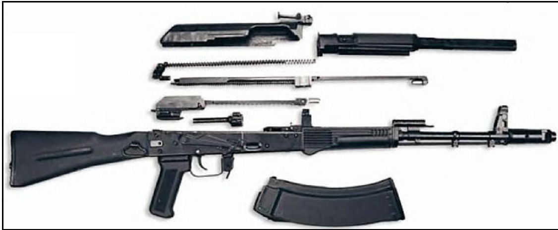
AK-107 assault rifle, disassembled
