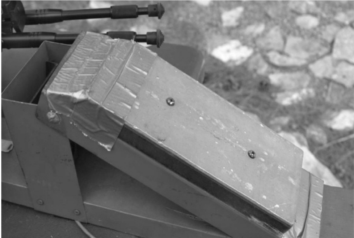
Full view of screen armor plate used to protect the photo cell system.
