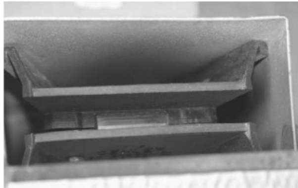
Top view of a Chronotech Model 33 sky screen photo cell that measured the velocity of the bullet downrange. This very fragile system needs to be protected by heavy armor at all times.
