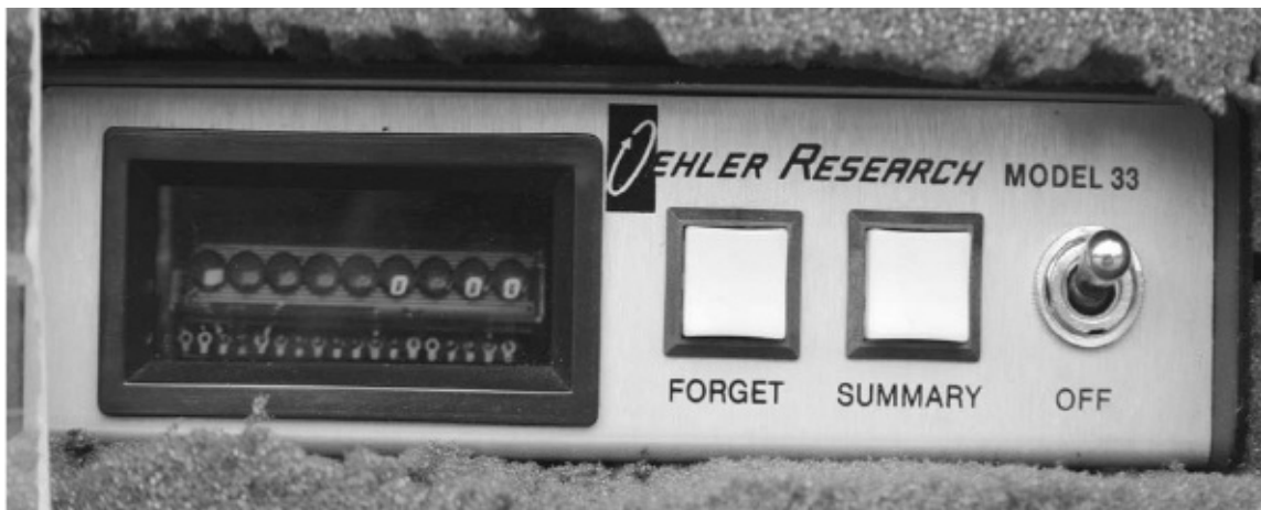
Front view of Oehler Model 33 Chronotech. This unit measured the exact velocity of a bullet at the muzzle, or at 400 yards downrange.
