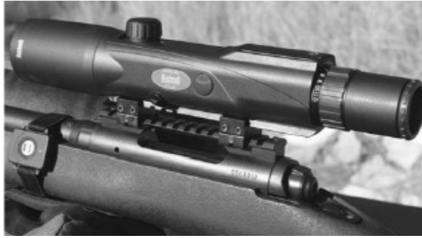
Bushnell Yardage Pro ranging scope. Note forend control wireless system used to activate the scope's ranging unit.
