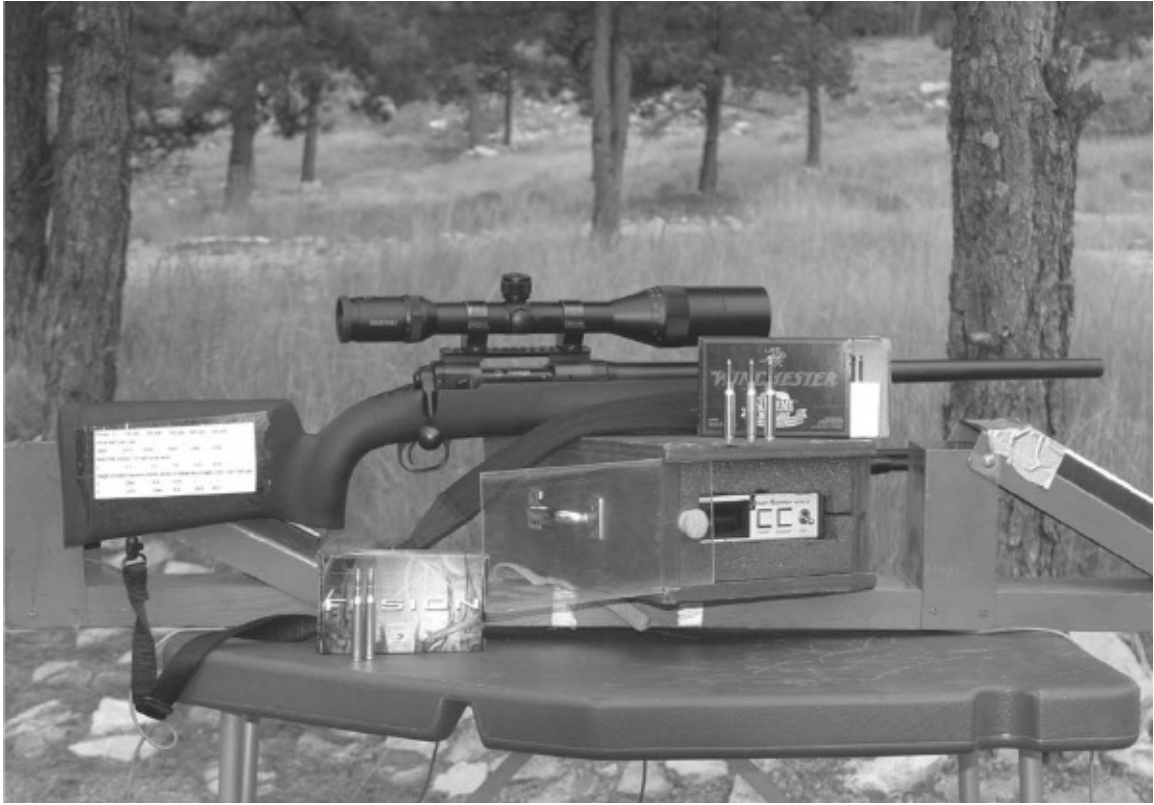
Author's chronograph unit and rail as used downrange for detailed bullet measurements.
