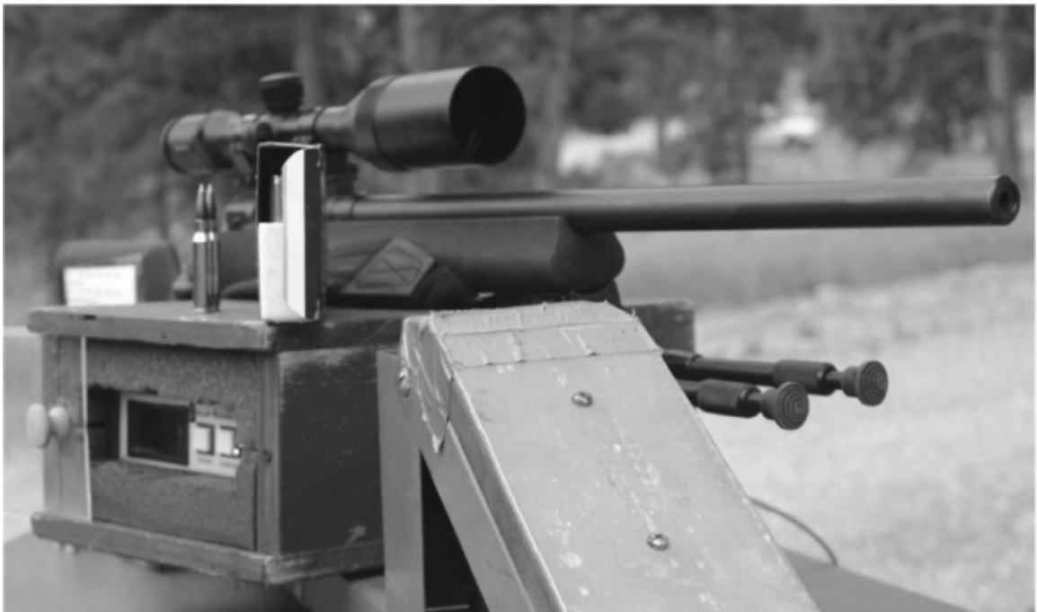
Savage Model 10 LE police sniper rifle is used for downrange work because it is accurate and gets bullets over those very small photo cell windows.
