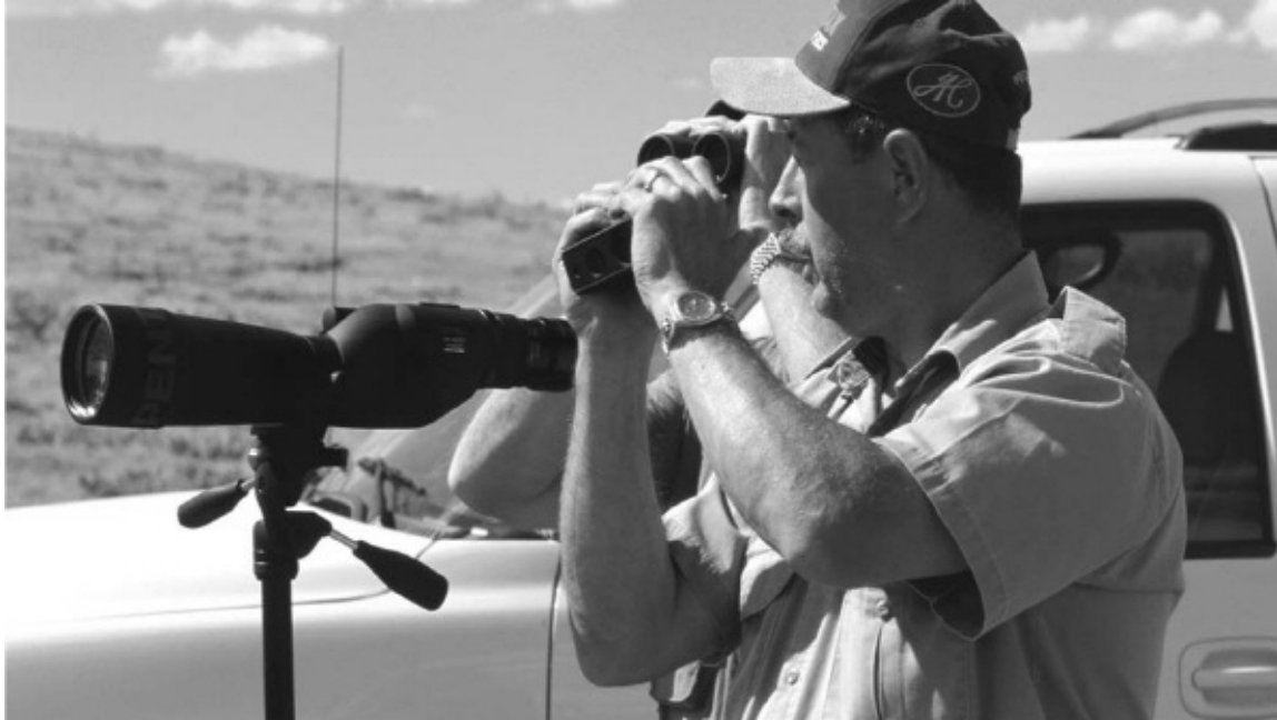
Leica rangefinder in conjunction with a spotting scope is being used here in the field. Multiple optics are often required when gaining exact and accurate information regarding range or hits on targets.
