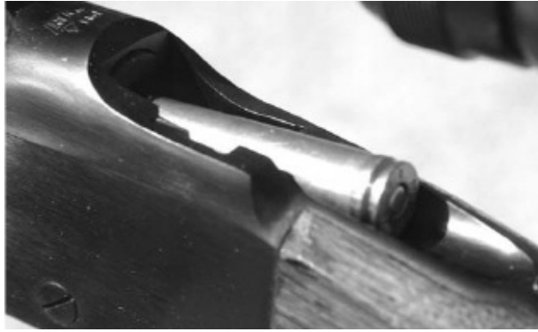
7mm Rem Mag in the loading gate of the Ruger single shot rifle.
