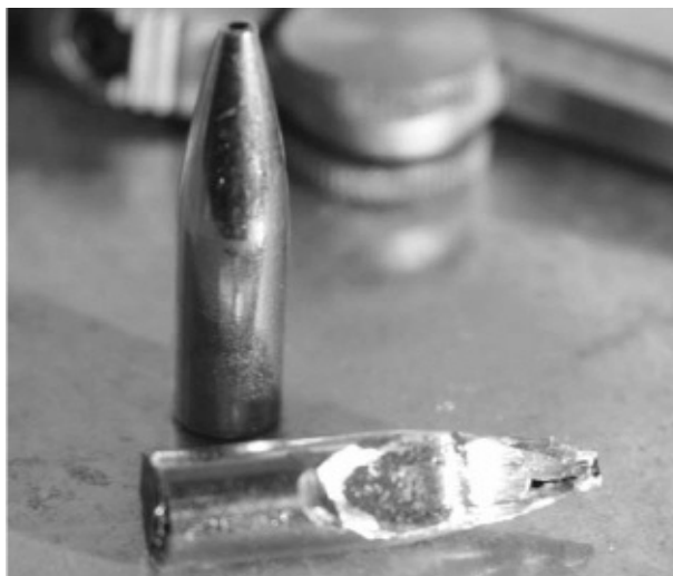
Dead Coyote bullet cutdown. Note the dust core at the center of the jacket.
