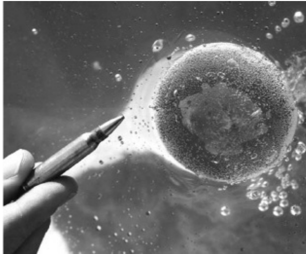
Dead Coyote 223 Rem handload being tested against dye-filled Perm Gel ballistic gelatin.
