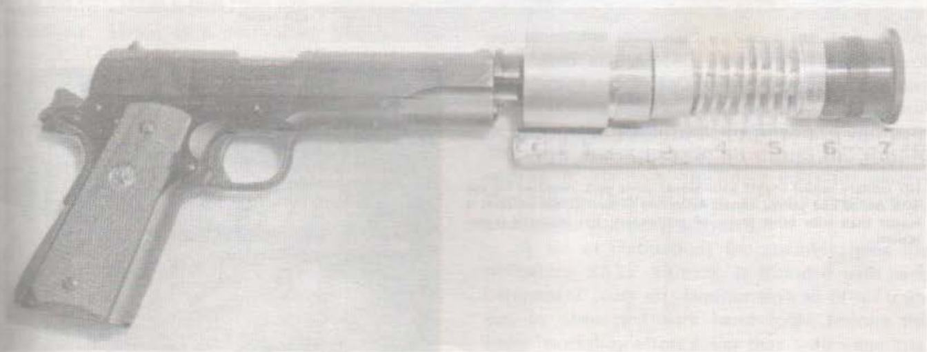
R. F. P.'s super mini kit and adapter bushing installed on a .45 government model.
