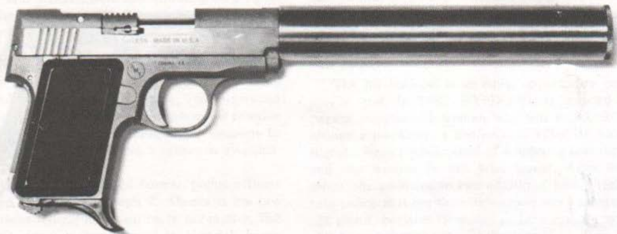
A New Jersey heroin dealer lost this prize when federal folks shut down his supply operations. Tests showed a drop of 28 dB with this unit attached.
