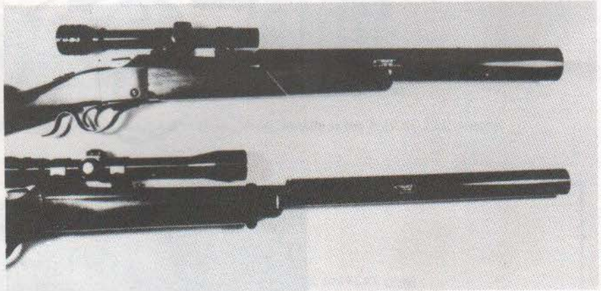
Dater also does custom suppressors. At top is an R3A custom unit on a Ruger No. 3 in .45-70, an integral unit. Bottom is a .223 muzzle suppressor.
