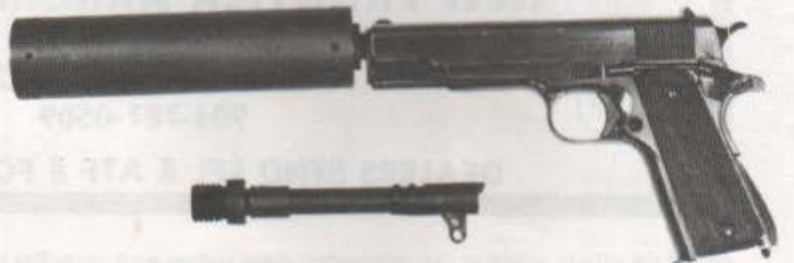
Colt .45 shown with long barrel made to adapt the MAC suppressor to it.
