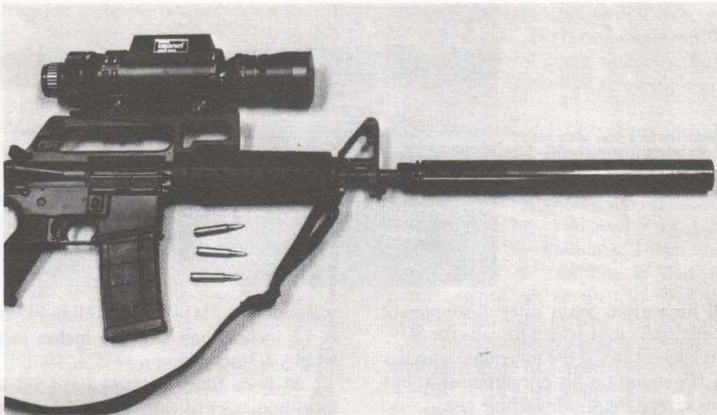
A Dater M22 suppressor mounted on an M16 with a Javelin night vision device.
