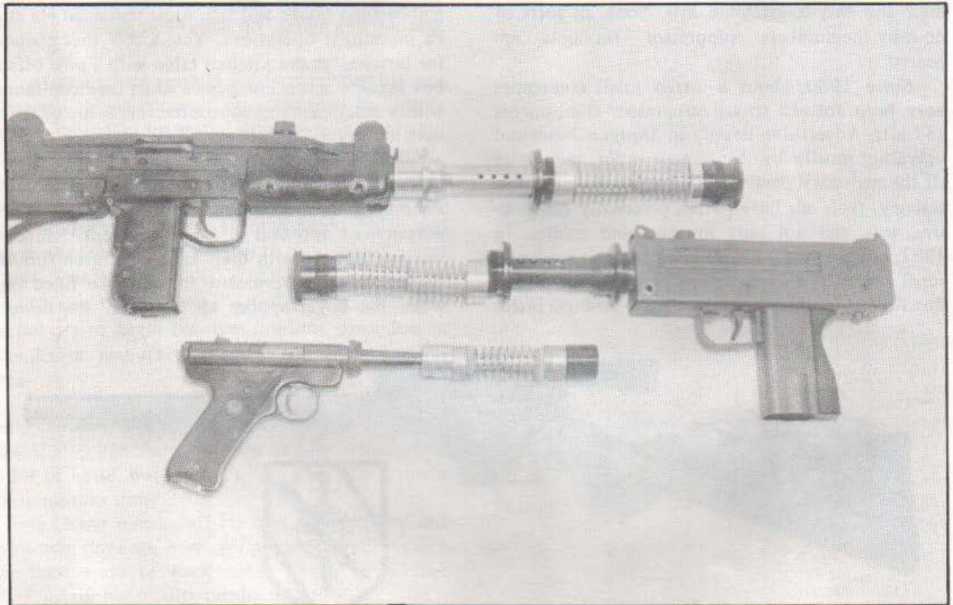
R. F. P.'s Uzi kit, the MAC 10 kit, and the Ruger RST 4 kit. Their Uzi design is unique in that the suppressor kit slides over the short barrel, replacing the barrel nut, which keeps the overall length to a minimum.
