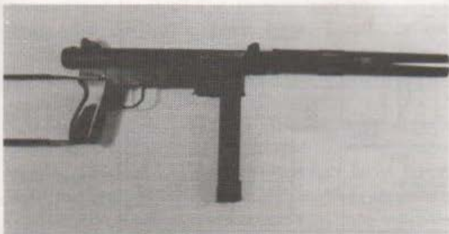
Phil Dater has standardized his 9mm suppressor as the SG9, adaptable to any 9mm submachine gun. It's shown here on a S & W M76.
