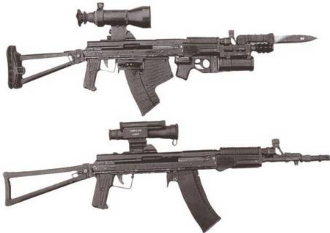
One of ASM-DT assault rifle prototypes, with underwater magazine and additional equipment (above) and with standard "above water" magazine (below)
