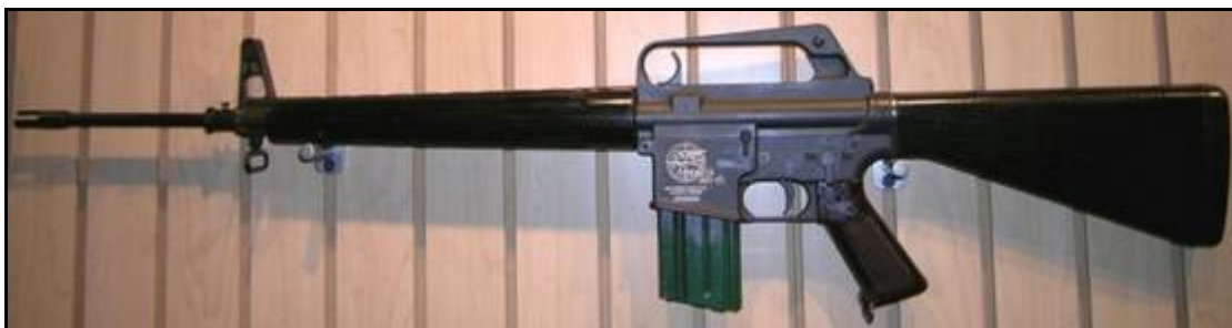
First model ArmaLite Ar-15 rifle, with original 25-round magazine. Note the position of charging handle
