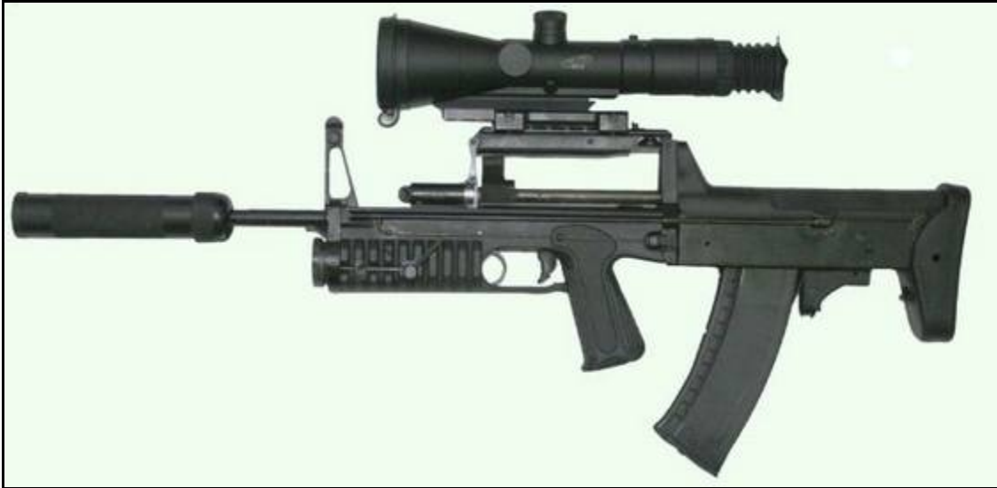
ADS dual-medium / amphibious / underwater assault rifle configured for above-water "Spetsnaz" use; grenade launcher barrel is removed, and a silencer and night sight are installed for special operations
