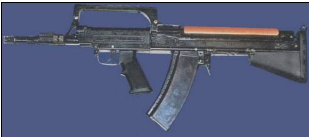
early prototype of the ADS dual-medium / amphibious assault rifle configured for above-water fire, with standard AK-74 magazine loaded with 5.45x39 ammunition
