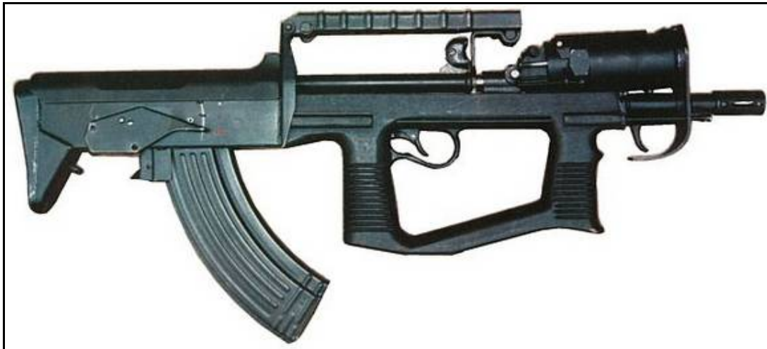
7.62mm prototype A-91 bullpup assault rifle, as made in mid-1990s. The integral 40mm grenade launcher is mounted above the barrel
