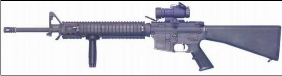
M16A4 rifle with RIS (Rail Interface System) installed around the barrel, and the Aimpoint red-dot sight installed on the rail instead of the detachable carrying handle
