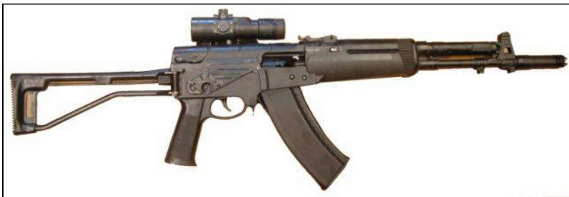
late production model AEK-971 rifle in 5.45x39mm with red-dot sight
