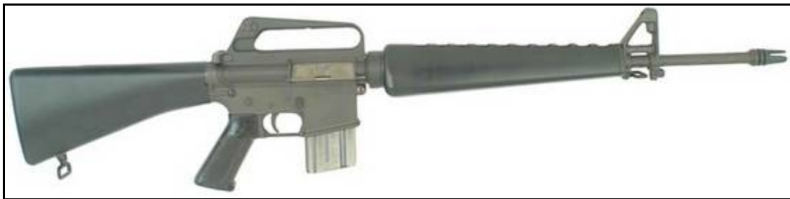
Early model M16 rifle, as used by US AF, with early military issue 20-round magazine. Note the three-prong flash hider and the lack of forward assist
