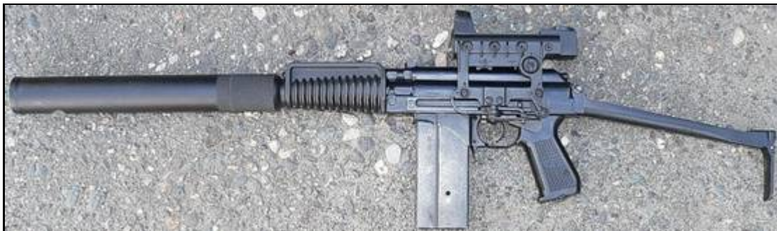
9A-91 compact assault rifle (current production model) with attached silencer and red-dot sight
