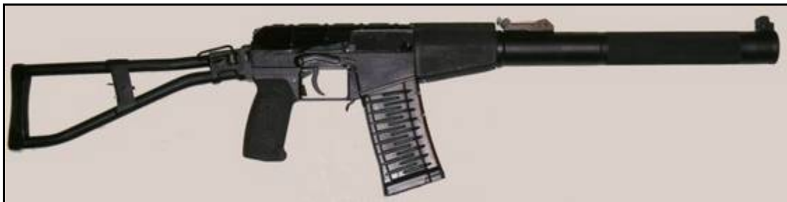
AS "Val" silenced assault rifle, with shoulder stock opened
