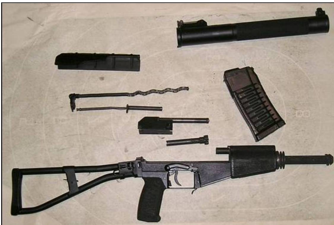
AS "Val" silenced assault rifle, partially disassembled; note that barrel is significantly shorter than integral silencer
