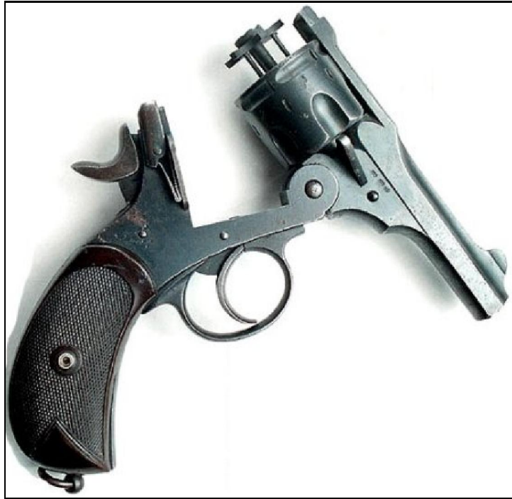
Webley .455 caliber MK. IV (Mark 4, 1899), frame broken open and extractor exposed from the cylinder
