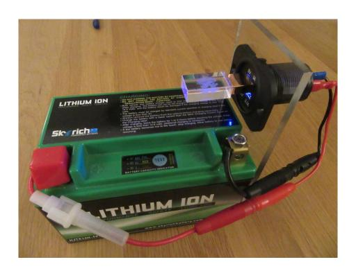
It is a 12V Lithium Ion battery and a 5V USB adapter. It appears to be an ideal power supply for the 5G key.
