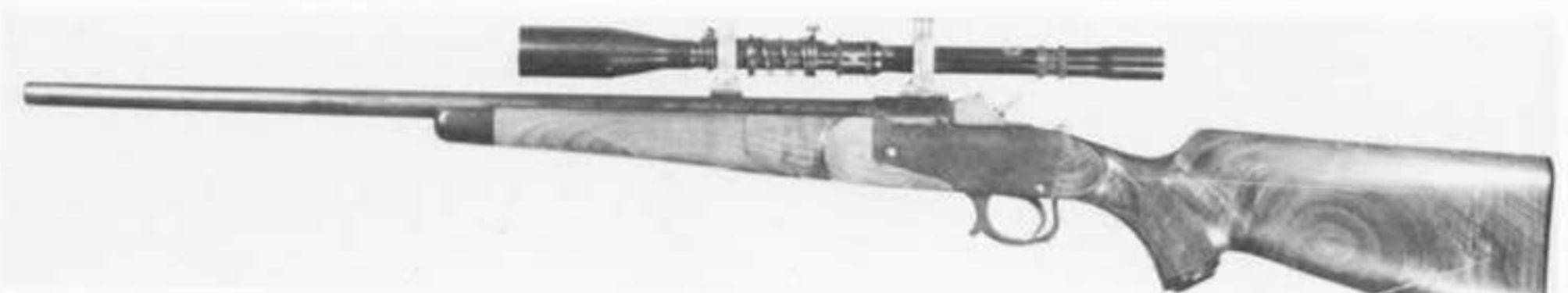
Fig. 1-7 This is the larger centerfire version of our CHICOPEE design which we have designated the F.D.H. CHICOPEE C.F. It differs mainly from the rimfire action and rifle in that the rifle has a two-piece stock, heavier and stronger action and a different breech block locking mechanism. This rifle chambered for the .218 Bee cartridge has a 24'' round tapered barrel on which is mounted an obsolete Fecker Woodchucker 7X scope and weighs about 8 pounds.
