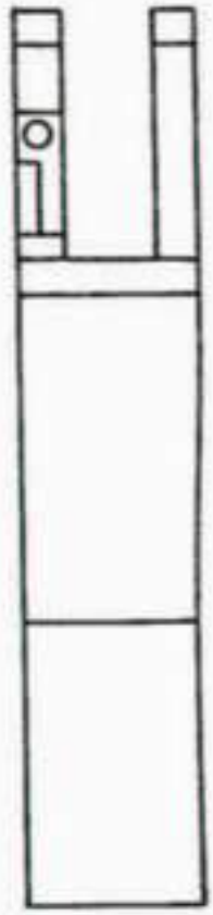
Fig. 3-11 FINISHED TRIGGER GUARD HOUSING This drawing shows side, top and front end views of the finished trigger guard housing. The finger lever spur is bent into the desired or required curve and need be only two-finger width in length. Make holes and pins for the hammer and trigger 9/64 " in diameter. Make the four small holes and pins 1/16 ". The lines on the right front end of the housing show the recess for the hold-close plunger, shown in detail in Figs. 3-25 and 3-26. The dotted lines at the rear of the hinge pin hole indicated by the letters TD show where metal has to be removed to make this hole a slot in order to make the action a quick take-down one as described at the end of this chapter.
