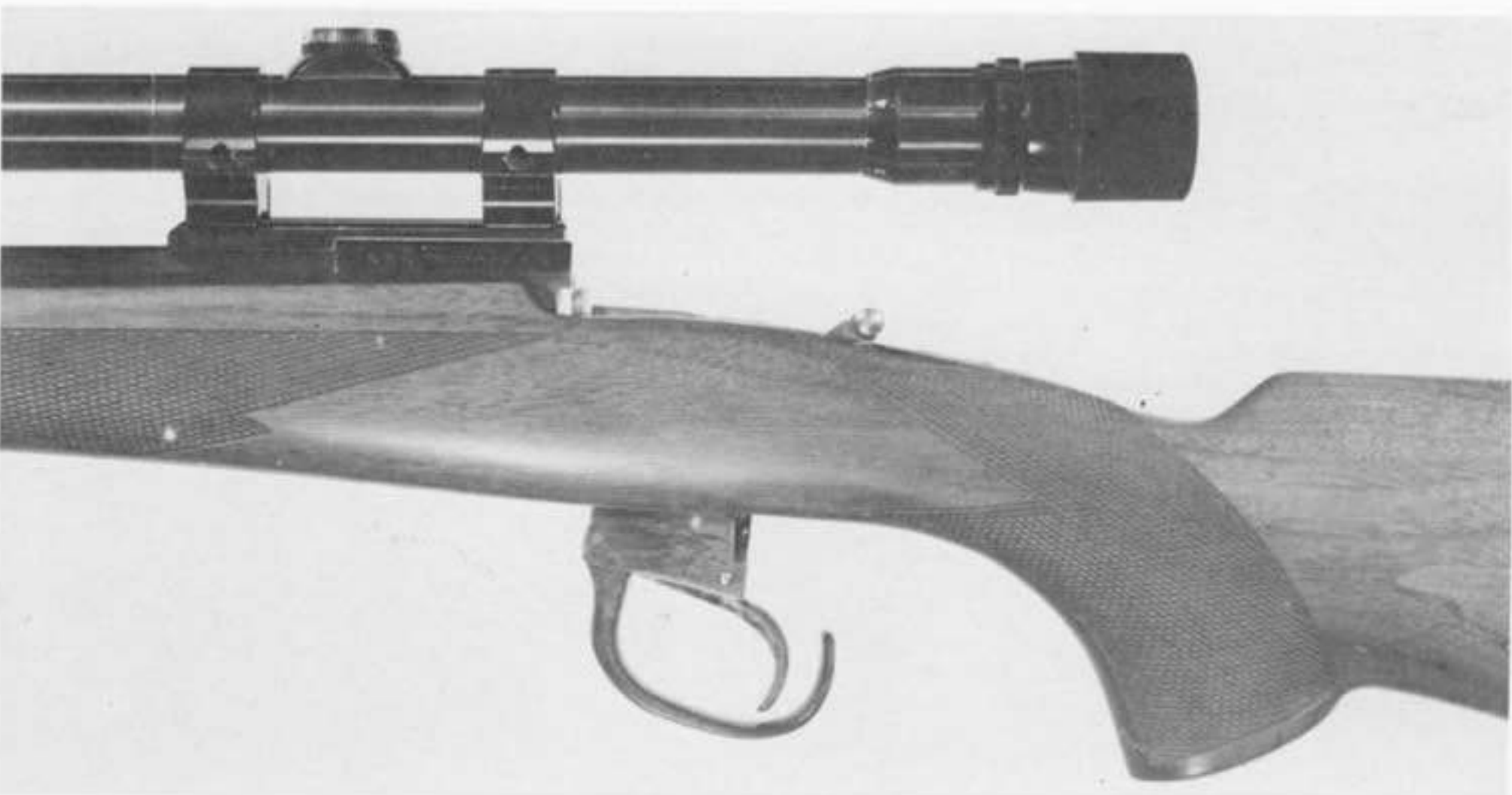
Fig. 1-6 Close-up of the F.D.H. CHICOPEE R.F. action showing it opened. A groove in the upper surface of the breech block becomes the loading platform to guide a cartridge into the chamber. The entire firing mechanism of this action is built into the sandwich constructed breech block which in turn fits between the sandwich sides of the receiver. To close this action you merely press upward on the trigger guard and when fully closed the locking latch shown behind the hammer flips forward to lock the breech block closed.
