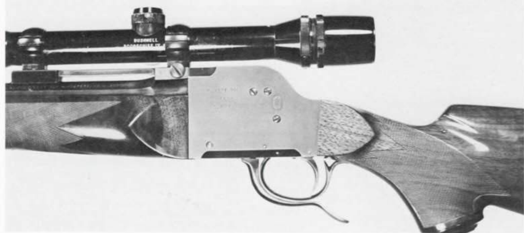
Fig. 2-B The left side of the FM No. 1 VAULT LOCK action. The upper two screws hold the hammer in place and the small oblong part is the sear/safety hold-down plunger. The lower screw is the sear/safety retainer screw. Two other photos of this rifle and action (Figs. 1-1 and 1-2) can be seen in Chapter 1.
