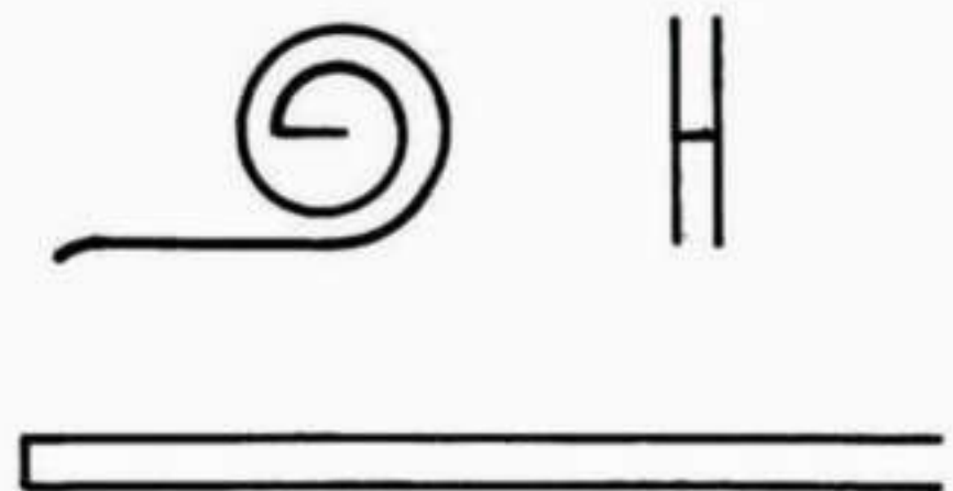
Fig. 4-16 ROTARY LOCK SPRING Side and end views of the rotary lock spring, plus a view showing the starting step in forming the spring. (Also see Figs. 4-1 and 4-2.)
