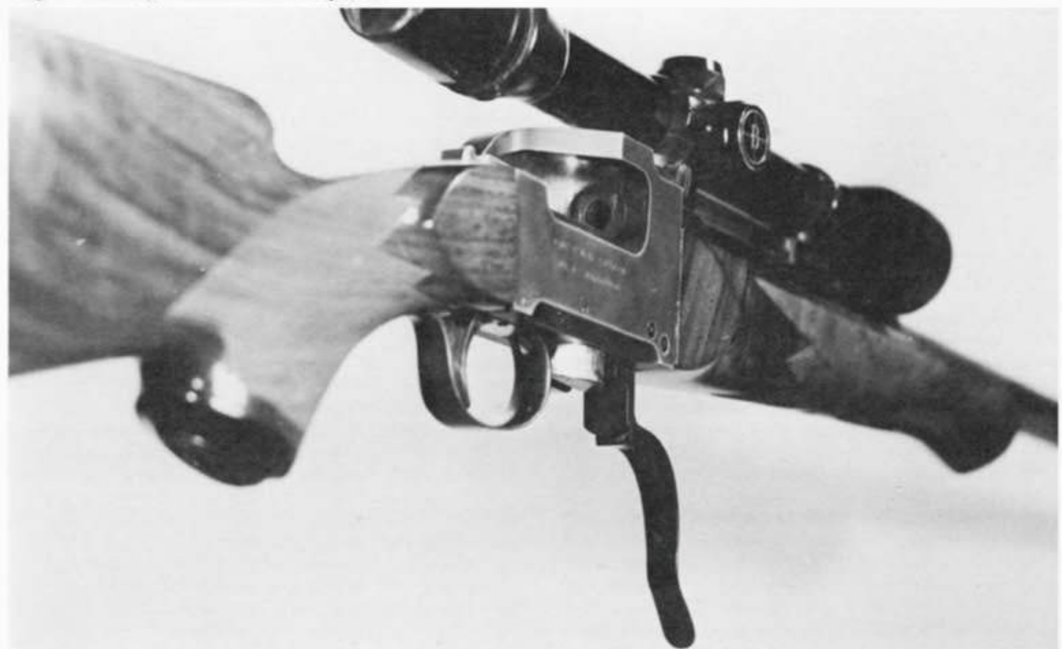
Fig. 2-C A close-up of the opened action of the rifle in Fig. 2-A. The name VAULT LOCK was chosen for this action as it describes the appearance and movement of the breech block since it is not unlike a cylindrical locking bolt in an ordinary bank vault door. The hammer must be manually cocked before the action can be opened and on being cocked it is automatically put on SAFE, and in addition, locked there so that it cannot be released while the action is open.
