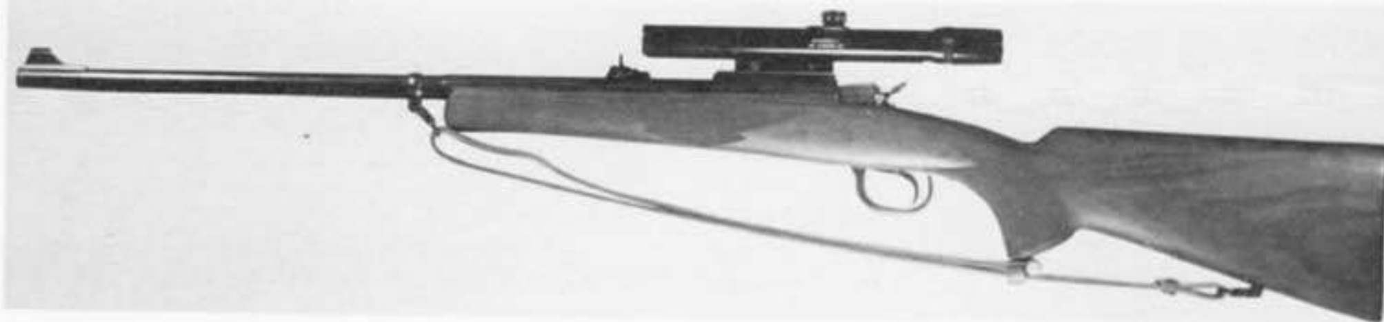
Fig. 1-5 An F.D.H. CHICOPEE R.F. rifle chambered for the .22 Long Rifle cartridge ready and fully equipped with sling and scope for the small game hunter. This was our prototype model with a 23'' half octagon barrel, 4X Bushnell scope, Jaeger 7/8'' carrying sling and auxilliary open sights.
