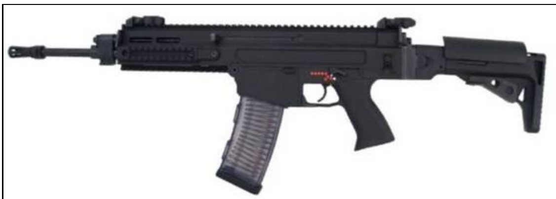
CZ 805 BREN A1 assault rifle with standard barrel
