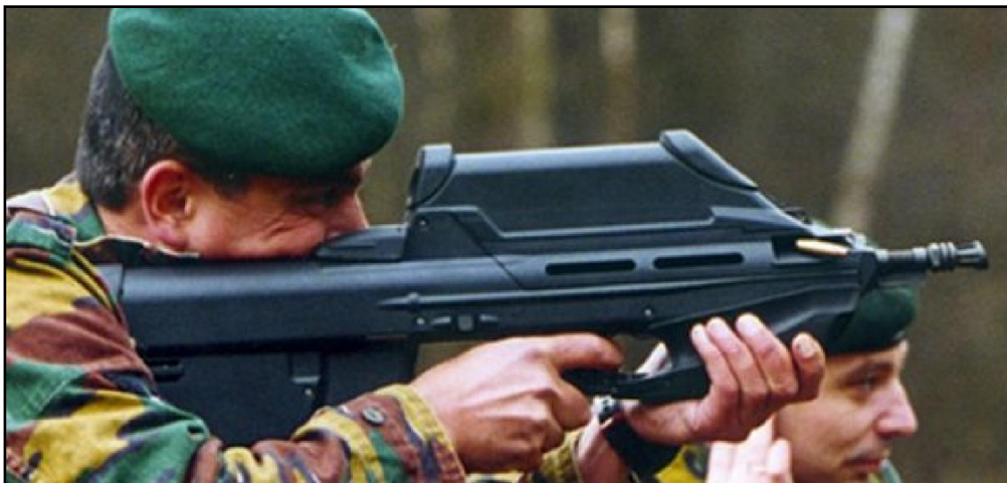
FN F2000 rifle being fired by Belgian soldier. Note spent case emerging from the port at the front of the rifle
