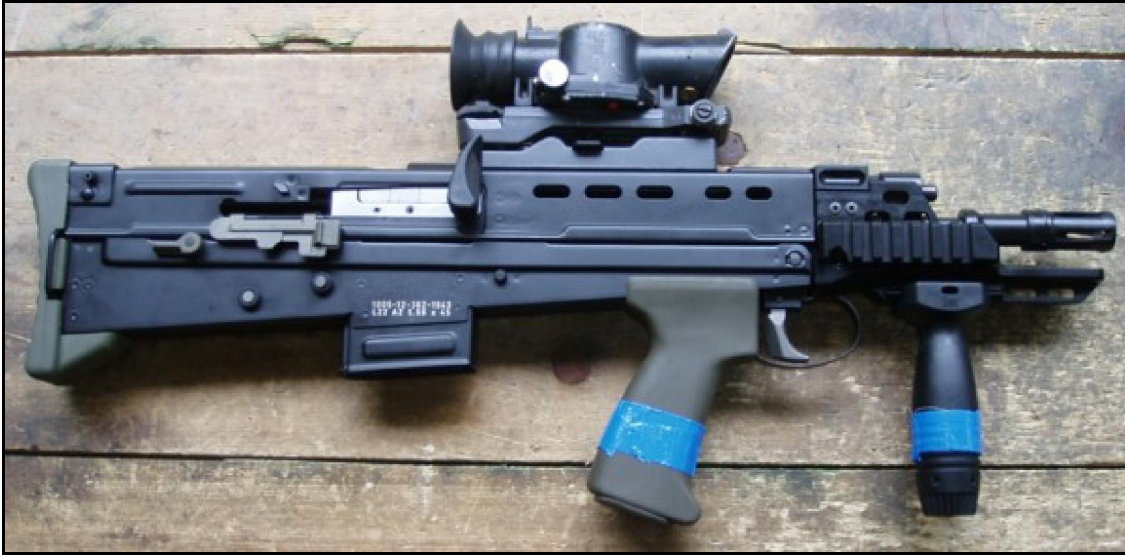
L22A2 carbine, as issued to Royal Armoured Corps tank crews in Iraq; note that it has a Picatinny rail above the front grip
