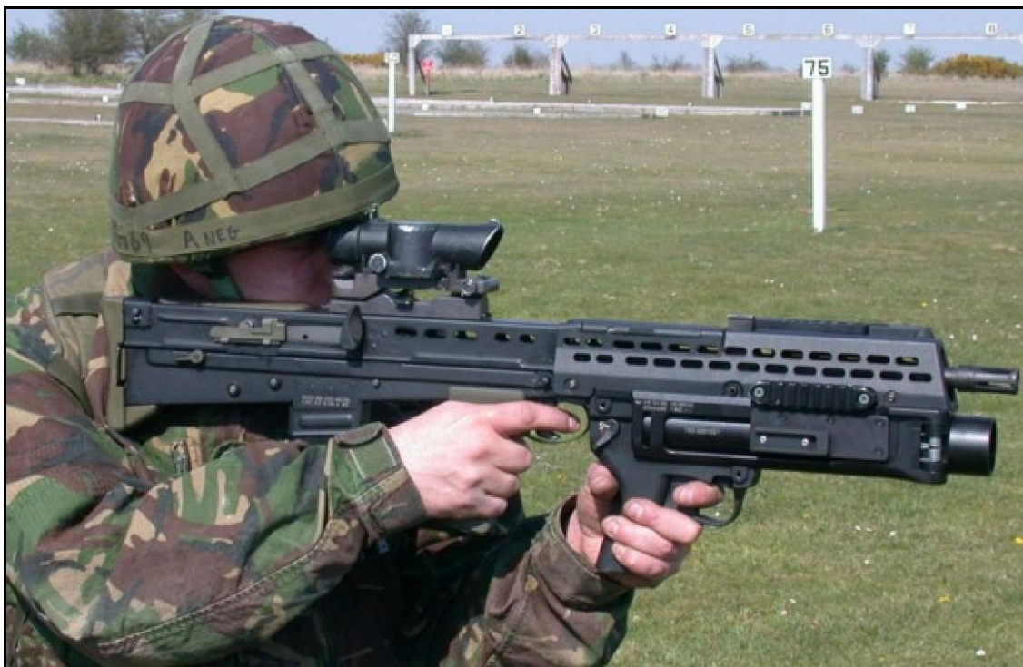
British soldier sights the L85A2 rifle fitted with German-made 40mm grenade launcher
