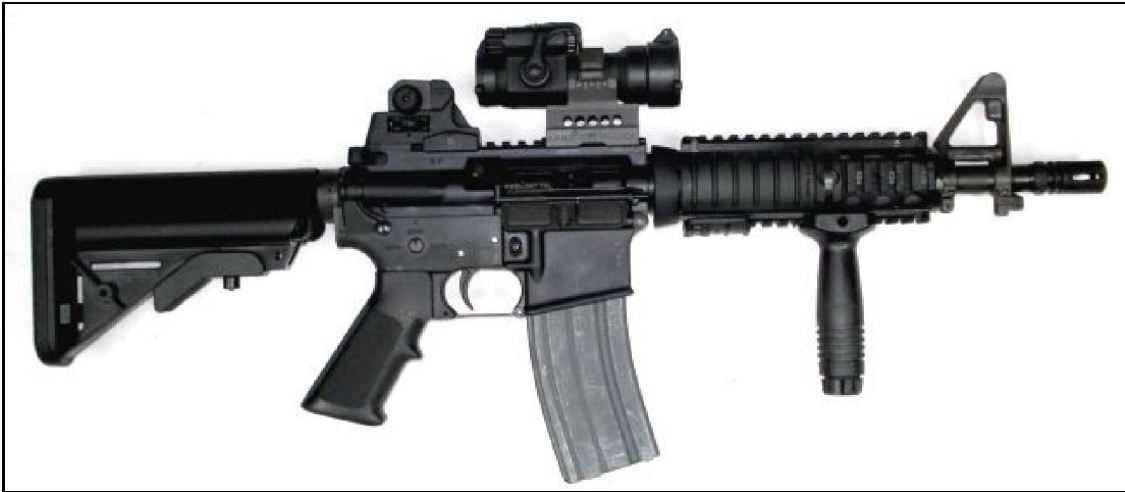
Colt M4 carbine with Mk.18 CQBR upper receiver, fitted with Aimpoint red-dot sight and additional back-up iron sights (BUIS)
