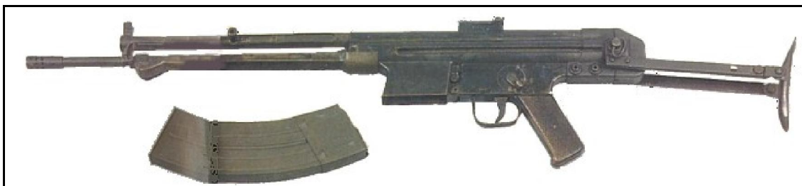
Early CETME assault rifle prototype chambered for experimental 7.92x40mm cartridge
