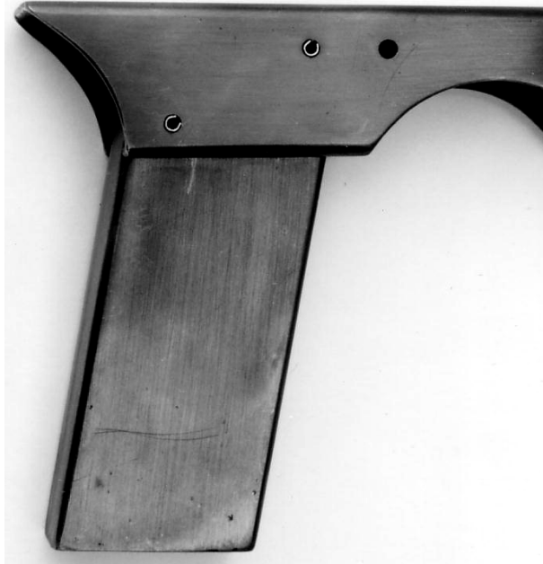
Photo 6: The grip pinned in position
