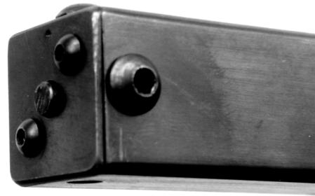
Photo 39: The recoil shield fitted to receiver.
