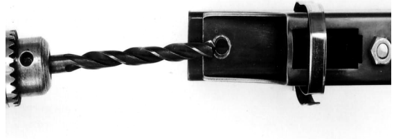
Photo 24: Drilling through the lower receiver bolt holes.
