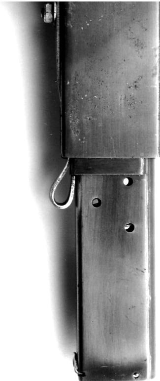
Photo 15: The spring catch holding magazine in place.
