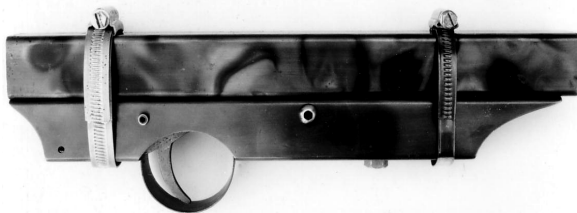
Photo 23: The receivers are clamped together with two hose clips.
