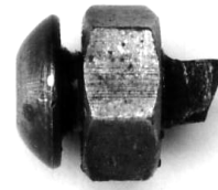
Photo 35: The Ejector Bolt and nut.
