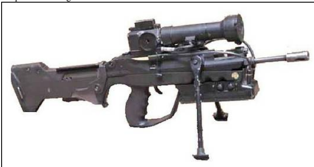
FAMAS-FELIN system prototype (2001). Modified FAMAS G2 rifle fitted with electronic day/night optical sight, laser rangefinder and an interface to the other soldier equipment, such as helmet-mounted display (HMD).
