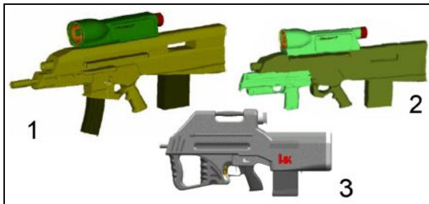
Some of the early OICW configuration alternatives (late 1990s). 1 - combined 5.56mm rifle and 20mm launcher (present configuration); 2 - 20 mm launcher with detachable 4.6mm HK PDW submachine gun; 3 - 20mm launcher in the standalone configuration
