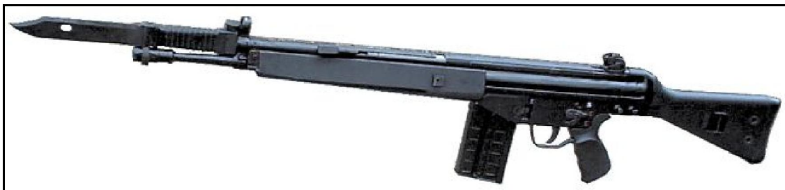
G3A3 with attached bayonet and plain plastic handguards of more modern appearance
