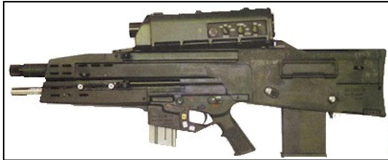
The left side view on the XM-29 OICW, showing its controls on the sighting unit
