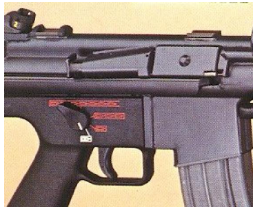
close-up view to the G41 receiver with dust cover, forward assist button and STANAG magazine well
