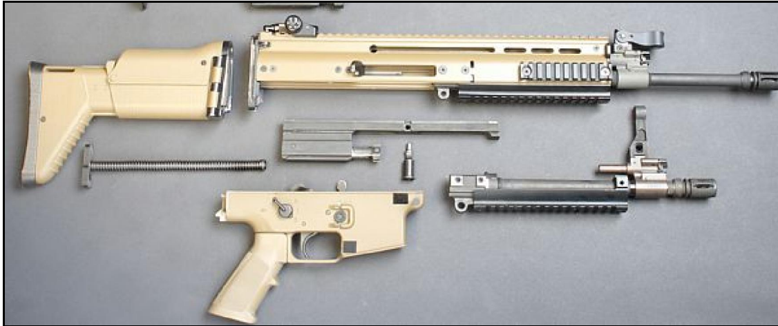
FN SCAR-L / Mk.16 rifle partially disassembled; note additional quick-detachable barrel
