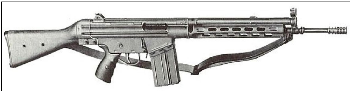
Earliest variant of G3 rifle with flip-up rear sight and metallic ventilated handguards
