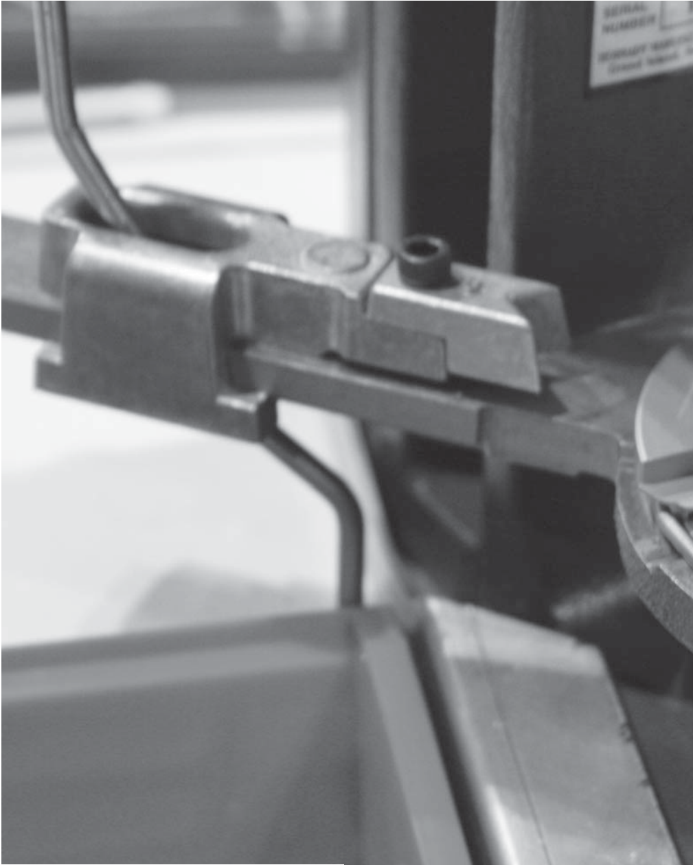
The Hornady case feeding mechanism, shoving another case into the shell plate.
