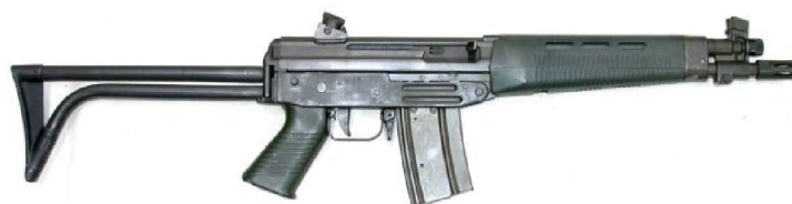
5.56mm SIG SG-543 short assault rifle, with side-folding butt
