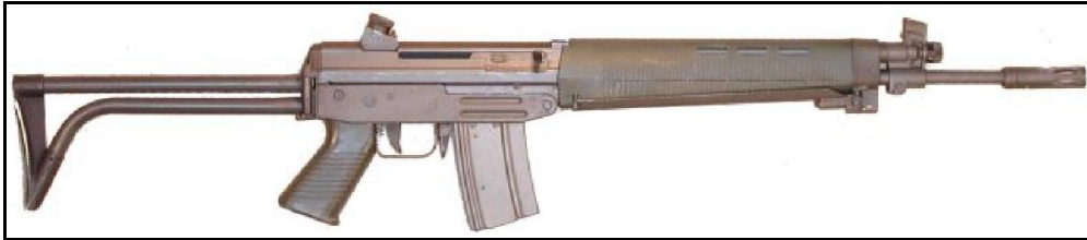
5.56mm SIG-Manurhin SG-540 assault rifle as made in France under license, with side-folding butt
