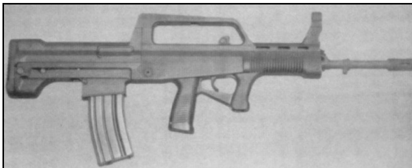
5.56x45mm QBZ-97 / Type 97 assault rifle; note different magazine port, designed to accept STANAG / M16-type magazines
