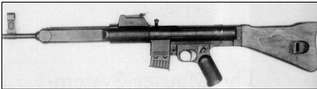
Mauser Gerat 06, an early roller-locked, gas-operated prototype dated to circa 1943
