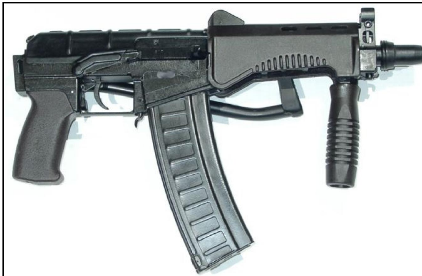
SR-3M Vikhr compact assault rifle, current issue model, with 'new pattern' 30-round magazine
