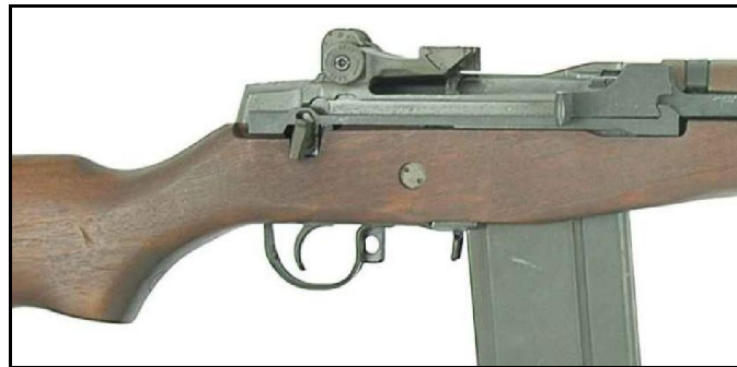
Close-up view on the controls of the military M14 rifle, including fire mode selector switch (on receiver above the trigger)
