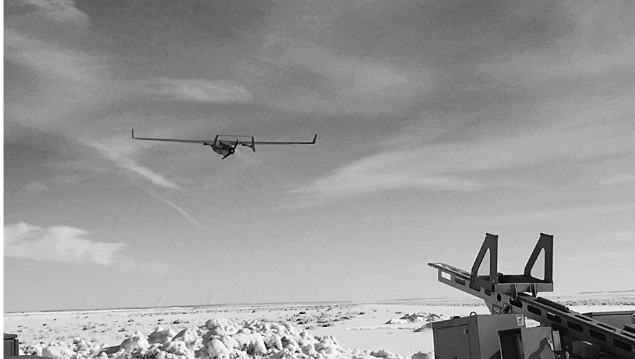
A Boeing Insitu Integrator catapult-launched drone equipped with Redkite, a miniaturized WAMI system, during testing in Boardman, Oregon, in 2017. Redkite is 40 times lighter than the early WAMI units, but just as powerful.
