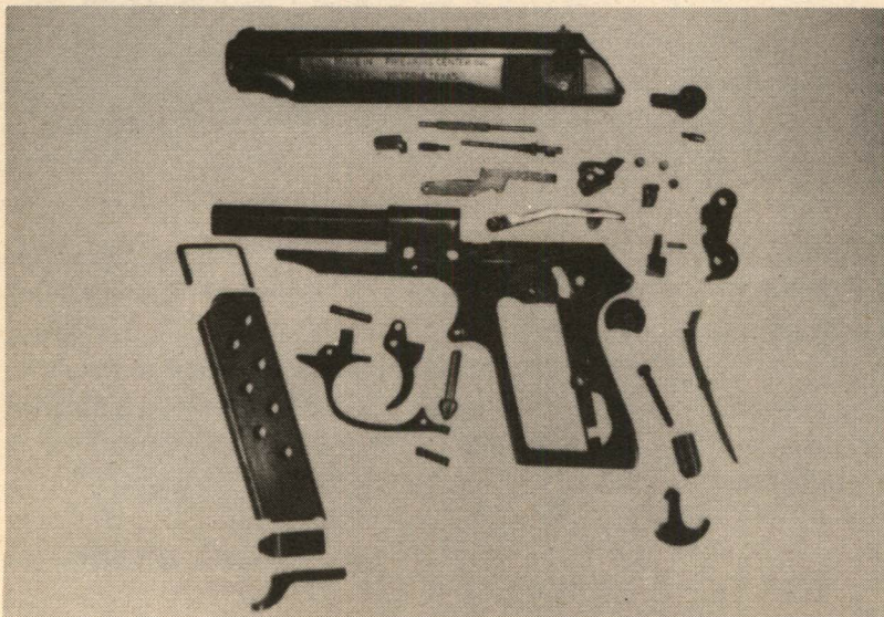
The MKE pistol, shown detail-stripped. Everything but the springs, ready to be sent to Armoloy.
