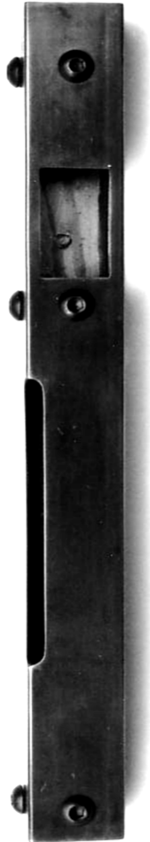
Photo 28: Three collars fitted to the receiver.
