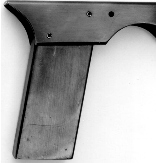
Photo 6: The grip pinned in position
