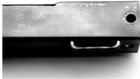
Photo 26: The Sling Loops are silver soldered in place.
