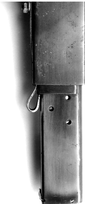
Photo 15: The spring catch holding magazine in place.
