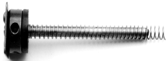
Photo 38: The recoil shield, mainspring and guide rod.
