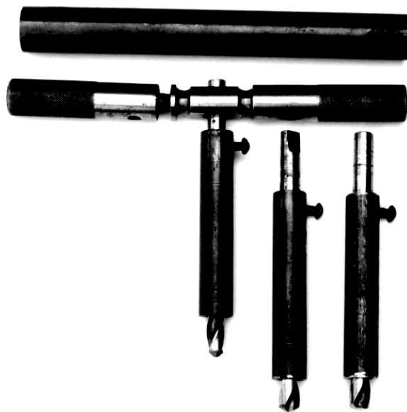
Note the flat ended No3 reamer tool; shown third from left.
